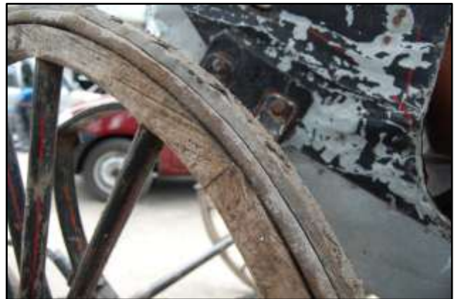
Figure 2: Wood used to construct the wheels in a hand-pulled rickshaw.
