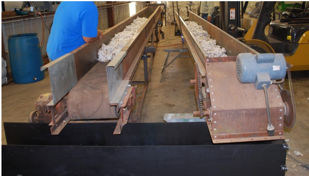
Figure 5. The two flow rate simulators used to control the material being conveyed onto the wire belt conveyor.
