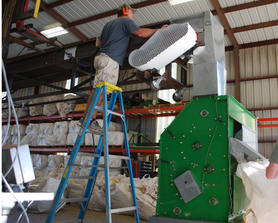
Figure 7. The flow rate simulator used to control the material being conveyed into the laboratory field cleaner.
