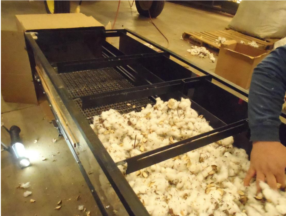
Figure 10. The guide marks on the divider were used to ensure the bur cotton bat was placed at the appropriate depth and can be seen on the right to the far end of the wire belt conveyor.
