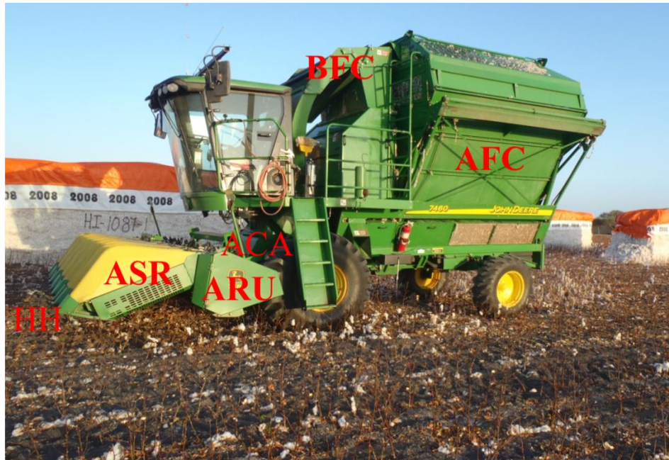
Figure 1. Collection locations for bur cotton samples represented on a John Deere 7460 cotton stripper similar to the one used.
