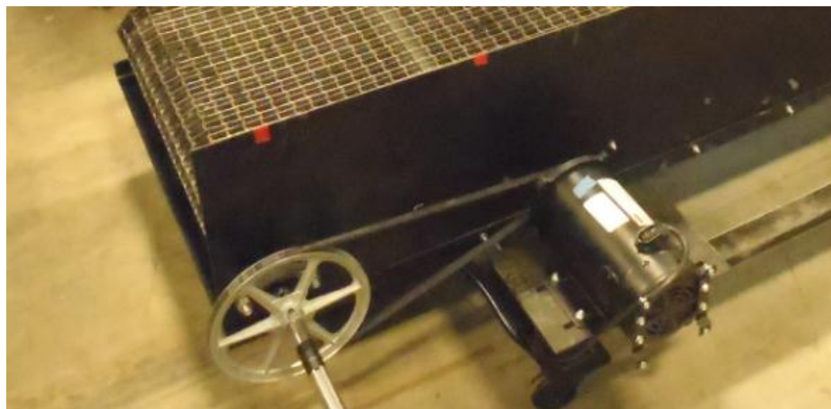
Figure 9. The motor and drive belt that operated the wire belt conveyor.
