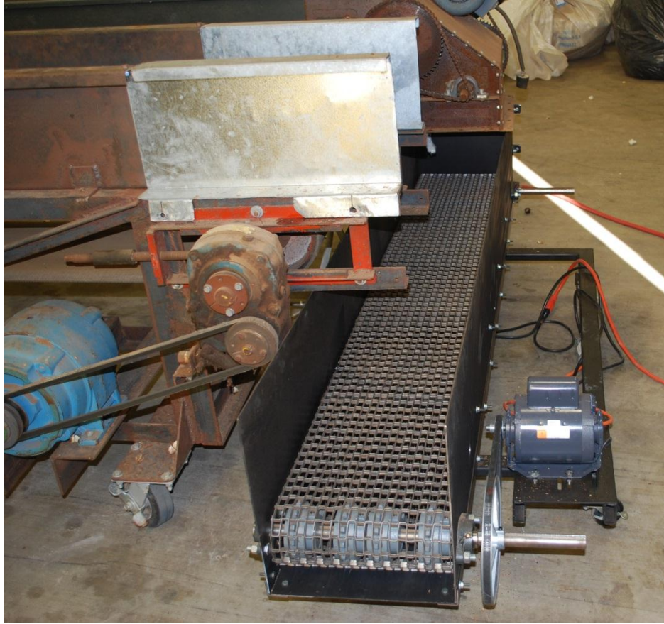
Figure 6. The wire belt conveyor used as a comparison to the cross auger.
