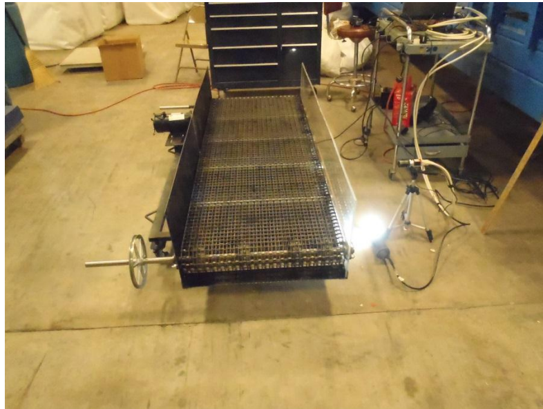
Figure 11. The high speed camera and the belt conveyor with the plexi-glass side installed.
