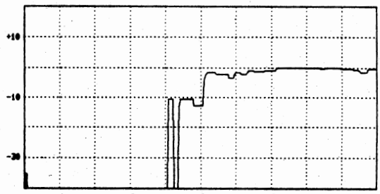
(c) SUPPRESSION FUNCTION (ATTENUATION [dB]) vs FRACTIONAL FREQUENCY; NOISE FILTER RESPONSE--SMOOTHED MAGNITUDE SUBTRACTION RULE
