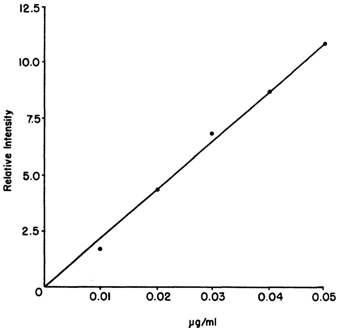
Figure 2. Relationship of relative fluorescence intensity to scopoletin concentration. Instrument, Aminco-Bowman spectrophotofluorometer. Photomultiplier, RCA 1P21 tube. Slit arrangement, 5. Light source, Xenon arc lamp. Meter multiplier setting, 0.3 and 0.1. Sensitivity setting, 0. Sample, aqueous 50% methyl alcohol from paper chromatogram. Activation wavelength, 365  $\text{m}\mu$ . Fluorescence wavelength, 468  $\text{m}\mu$ .
