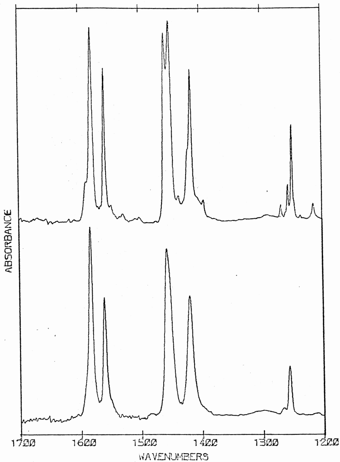
Figure 41. Spectra of "Glassy" Bipyridine at 77 K (Lower Curve), and of a Polycrystalline Film Obtained from Warming the Sample (Upper Curve)
