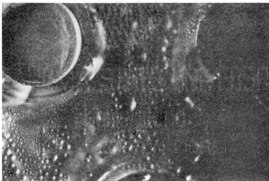
Figure 19. Visual Observation at Re=400 With 0.05 Inch Spacing
