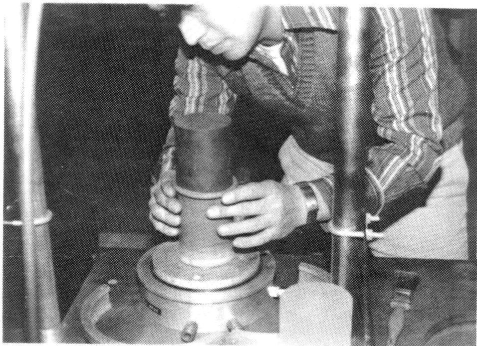
Figure 9f. Unrolling the O-Ring and Membrane to Enclose the Specimen
