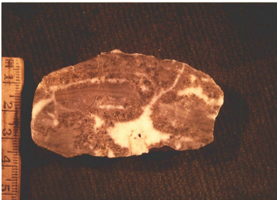
Fig. 15.-Sphalerite (yellow-brown), tectonic vein dolomite (white), and brecciated host rock (gray). Note that the brecciated host rock is laminated and that sphalerite does not coat all the visible sides. Also note that the tectonic vein dolomite cuts the sphalerite mineralization. (Scale is in cm.)
