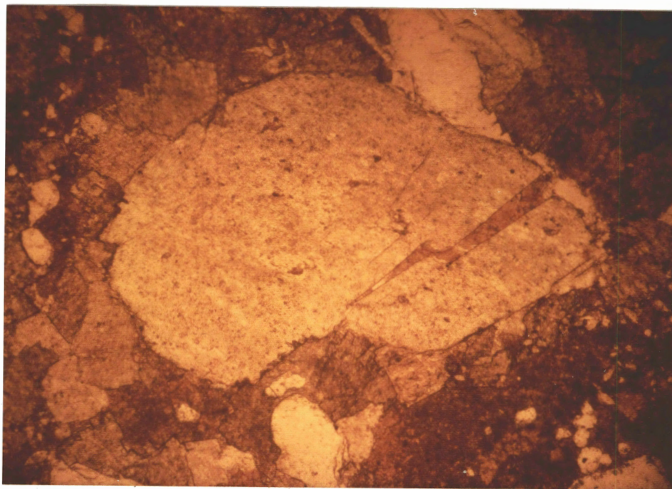
Fig. 11.-Fractured detrital feldspar with calcite (red) filling. Note that authigenic overgrowth (clear, upper-right) has closed the fracture. Dolomite (yellow) has replaced the feldspar in the lower left corner. 100X; stained with Alizarin Red-S and potassium ferricyanide; plane-polarized light.
