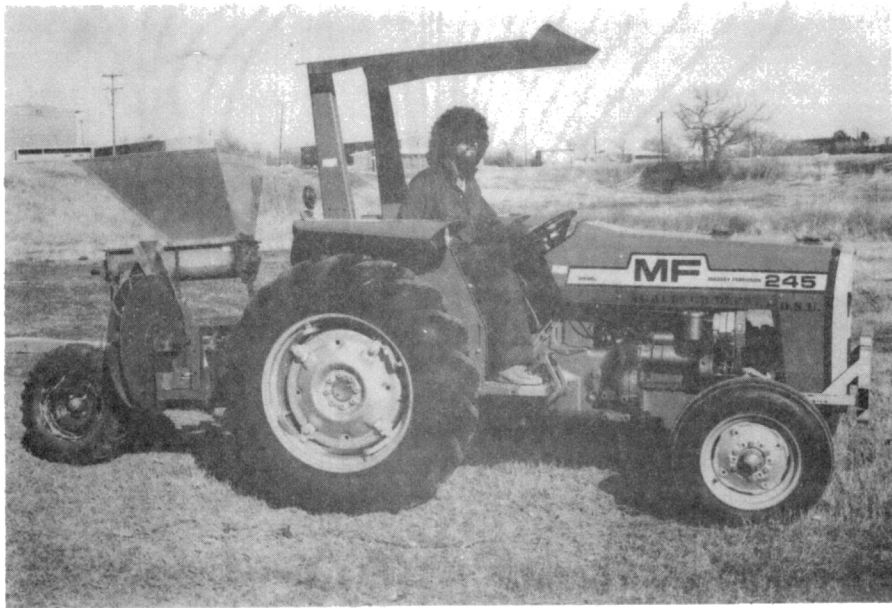
Figure 2. Side View of Vertical Distributor Connected to the Tractor
