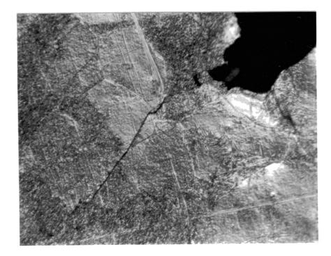
Figure 27. High Strain Amplitude Fracture Surface in a Dry Air Environment. In low cycle cycle fatigue the fracture surface has visible surface distortion with many grains having two or more slip directions. Sample 5B (X380)
