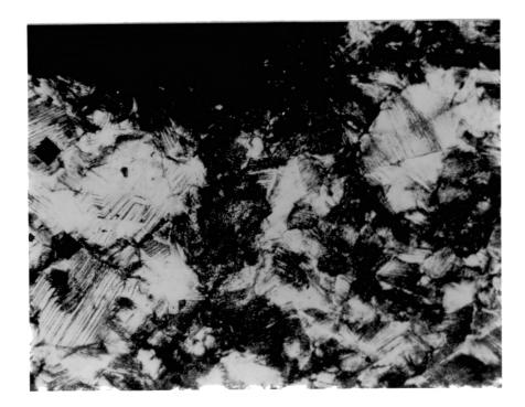
Figure 37. Example of Multi-Directional Slip. Grain in the middle has slip in three directions. Notice that adjacent grains of approximately the same orientation have slip in more than one direction. Sample was a preliminary test with a fatigue life of  $2 \times 10^5$ cycles in dry air. Sample (X190)
