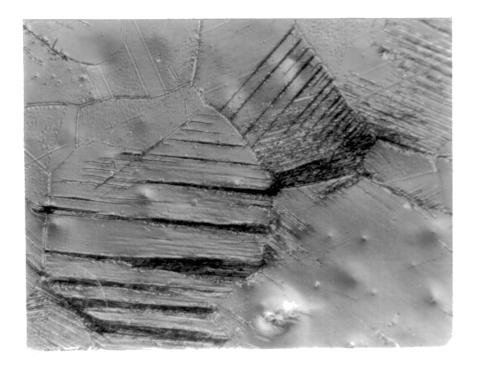
Figure 39. Stage I Crack Propagation. Cracking is in grains and along grain and twin boundaries. Sample is the same as in Figure 37 (X190)
