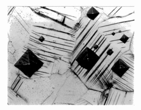
was found that the surface deterioration was often too great to get consistent hardnesses at the lowest load. This test load was eliminated and tests were made with the 50 and 500 g loads.
