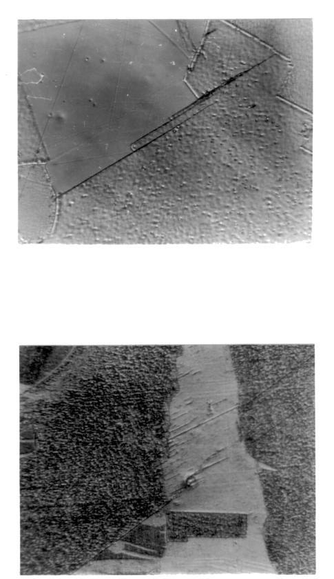
Figure 25. Low Strain Amplitude Fracture Surface in a Dry Air Environment. In the long fatigue life samples, the fracture edge has a distinct lack of gross surface deformation. Traces of slip are observed instead of distinct lines such as the crack along a grain boundary. Sample 4A (X380)
