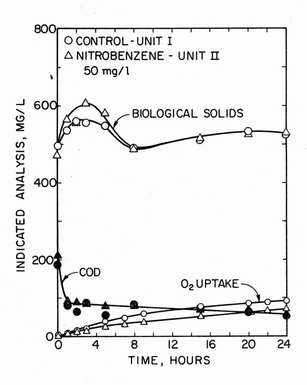
Figure 9. Performance of Unit I vs Unit II During 24-hour Batch Study on Day 114 at Beginning of Daily Switching of Nitrobenzene Dosage From 50 to 25 mg/l. Nitrobenzene Concentration - 50 mg/l
