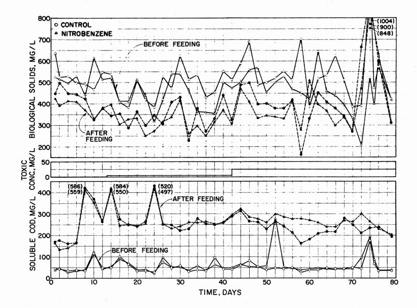
Figure 3. Performance of Unit I vs the Performance of Unit II From Day 79 to Day 158
