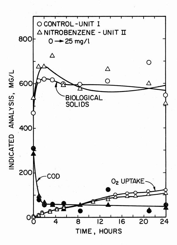
Figure 12. Performance of Unit I vs Unit II During 24-hour Eatch Study on Day 136 at End of Daily Switching of Nitrobenzene Dosage From 25 to 0 mg/1. Nitrobenzene Concentration - 25 mg/1
