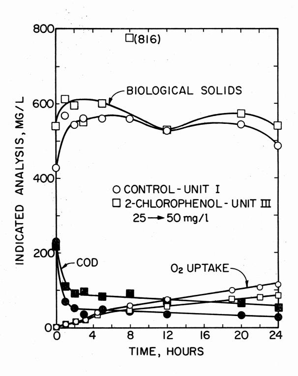
Figure 17. Performance of Unit I vs Unit III During 24-hour Batch Study on Day 122 at End of Daily Switching of 2-Chlorophenol Dosage From 50 to 25 mg/l. 2 -Chlorophenol Concentration - 50 mg/l
