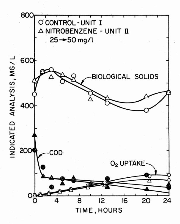
Figure 11. Performance of Unit I vs Unit II During 24-hour Batch Study on Day 128 at Beginning of Daily Switching of Nitrobenzene Dosage From 25 to 0 mg/1. Nitrobenzene Concentration - 25 mg/1
