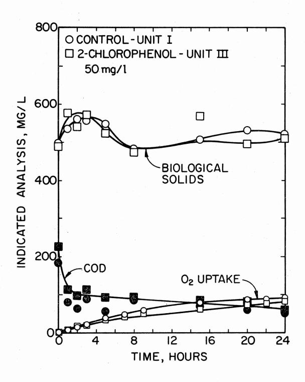
Figure 16. Performance of Unit I vs Performance of Unit III During 24-hour Batch Study on Day 114 at Beginning of Daily Switching of 2-Chlorophenol Dosage From 50 mg/l to 25 mg/l. 2-Chlorophenol Concentration 50 mg/l
