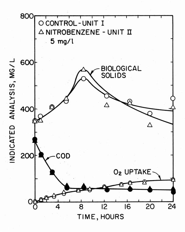
Figure 7. Performance of Unit I vs Unit II During 24-hour Batch Study on Day 42 First Day Unit II was fed 25 mg/l Nitrobenzene
