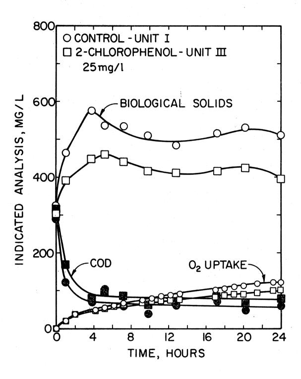
Figure 15. Performance of Unit I vs Performance of Unit III During 24-hour Batch Study on Day 81, First Day Unit III was fed 50 mg/l 2-Chlorophenol
