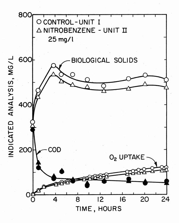
Figure 8. Performance of Unit I vs Unit II During 24-hour Batch Study on Day 81 First Day Unit II was fed 50 mg/1 Nitrobenzene
