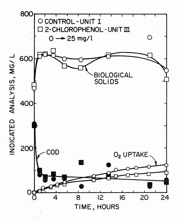
Figure 19. Performance of Unit I vs Unit III During 24-hour Batch Study on Day 136 at End of Daily Switching of 2-Chlorophenol Dosage From 25 to 0 mg/l. 2-Chlorophenol Concentration - 25 mg/l
