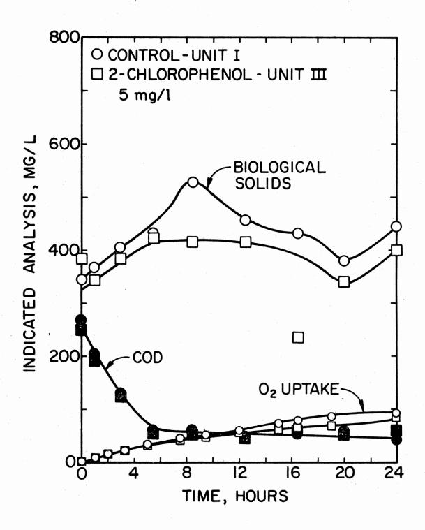
Figure 14. Performance of Unit I vs Performance of Unit III During 24-hour Batch Study on Day 42, First Day Unit III was fed 25 mg/l 2-Chlorophenol
