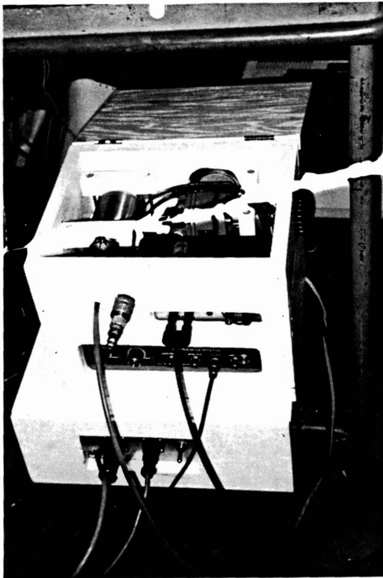
Figure I.3. Solenoid Valve Pulser (Top) and Stepper Motor Controller (Bottom)
