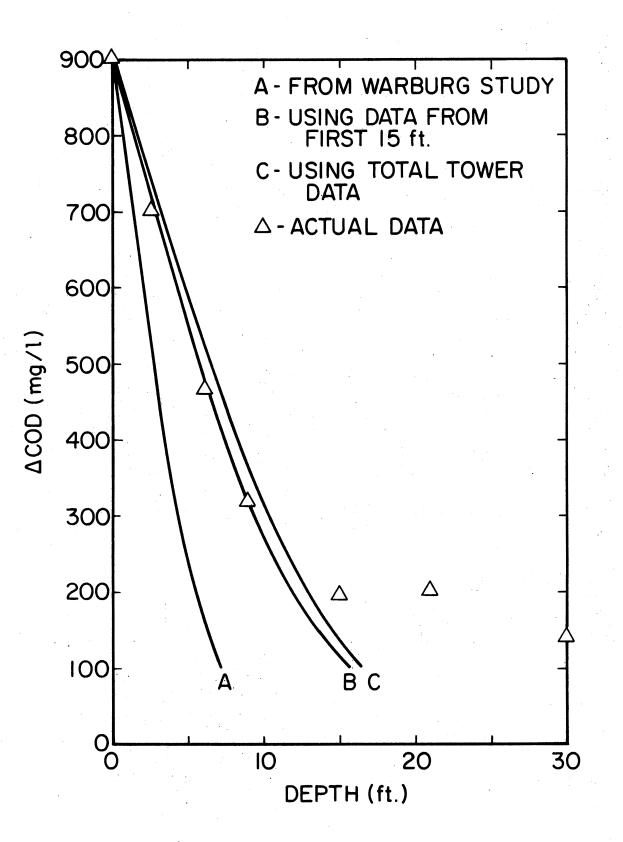
Figure 11. Theoretical  $\triangle$ COD Removal Compared to Actual Data at 850 gal/day ft<sup>2</sup>
