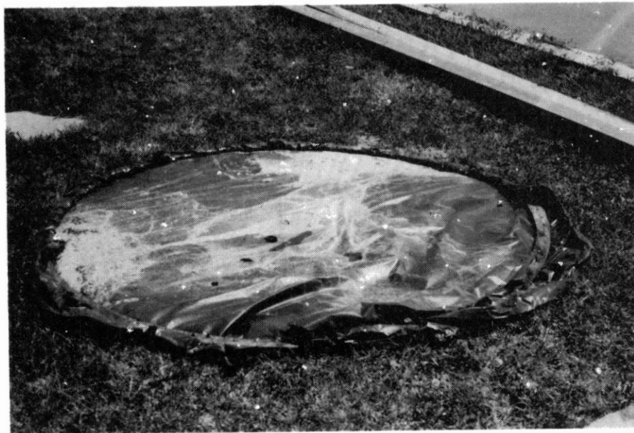
Figure 9. Condition of the Six Mil, Black Polyethylene After Deteriorating from the Ultra-violet Rays of the Sun
