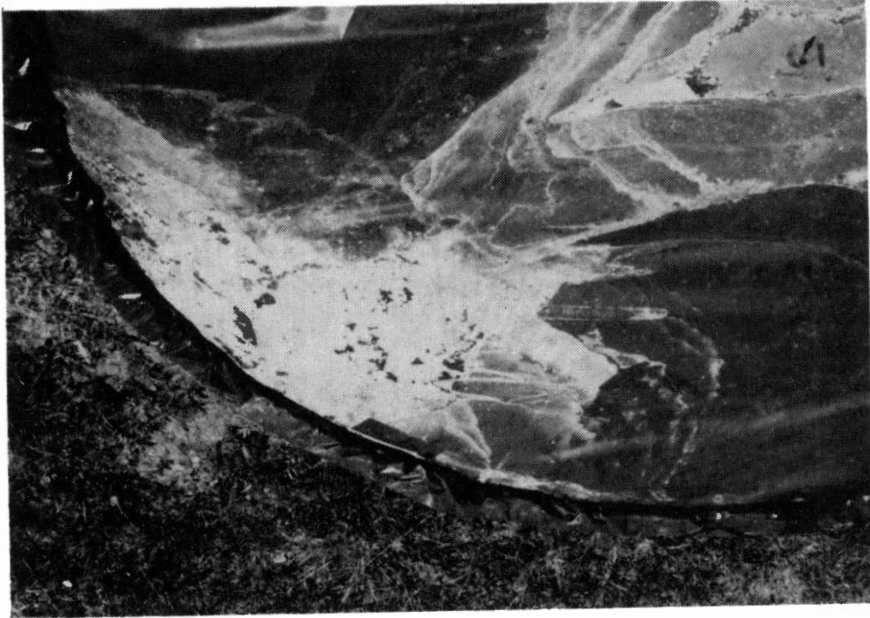
Figure 10. White-film Build Up on the Surface of the Six Mil, Black Polyethylene Absorber Surface
