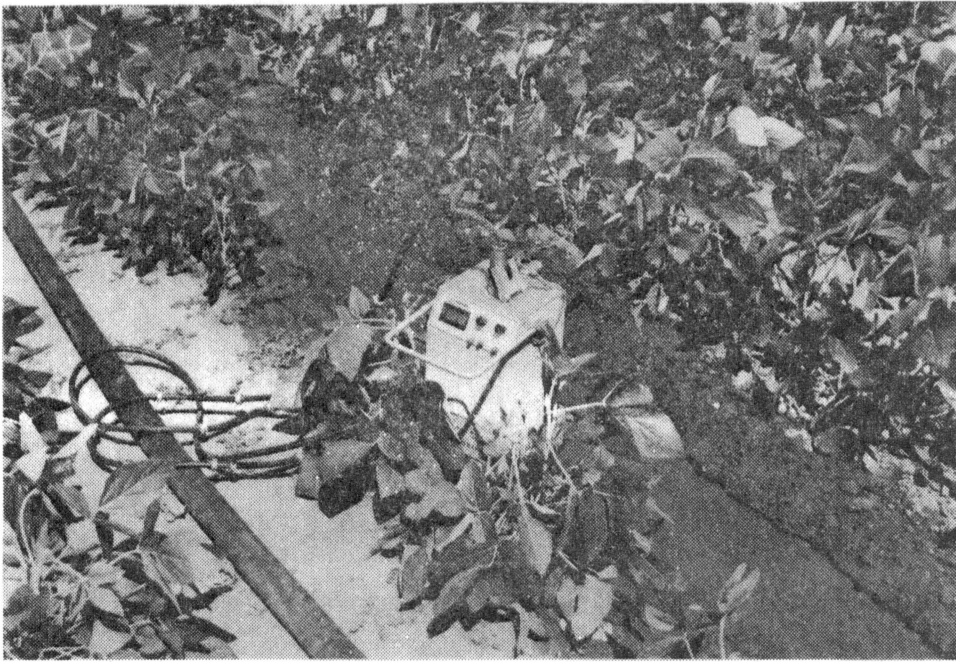
Figure 17. Neutron Moisture Meter at the Middle of the Infiltration Test Length
