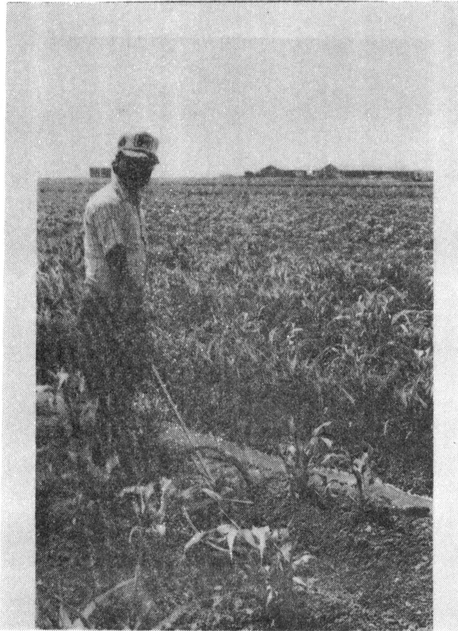
Figure 8. Measurement of the Advance Distance using an Odometer
