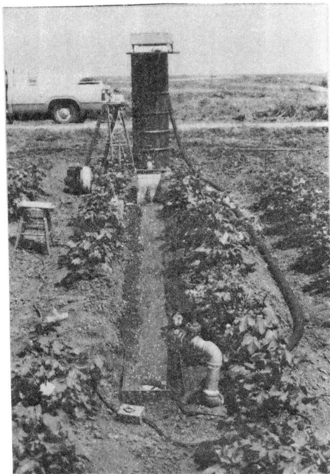
Figure 16. Blocked Furrow Infiltrometer in Field Operation
