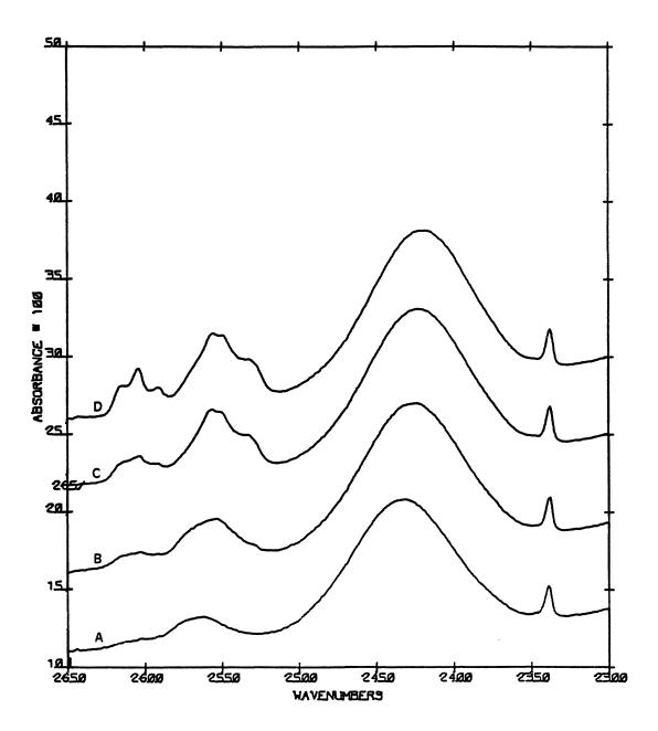
Figure 44. Hydrogen Sulfide Enclathrated with Some Conversion to Cubic Ice. A - 10 K; B - 15 K; C - 20 K; D - 25 K; and E - 30 K.
