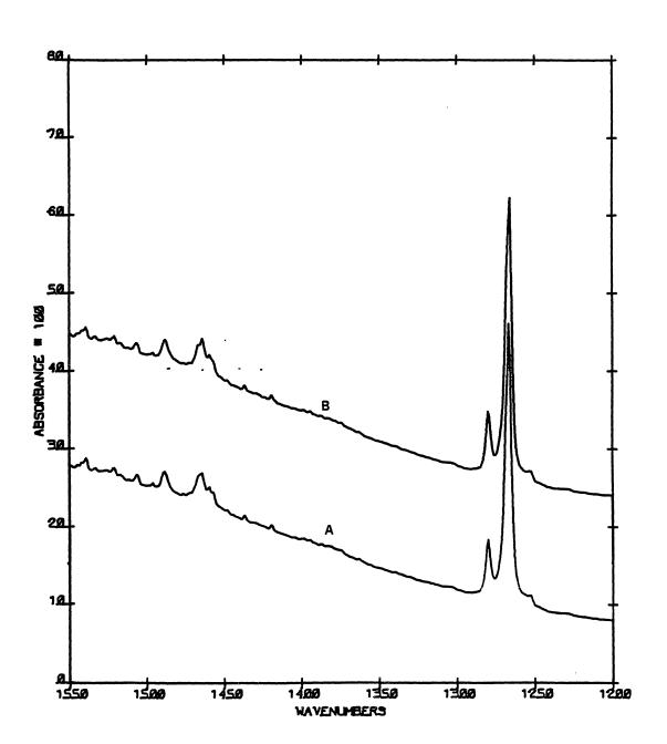
Figure 12. High Resolution  $(0.5 \text{ cm}^{-1})$  of Ethylene Oxide Clathrate Hydrate at 10 K.
