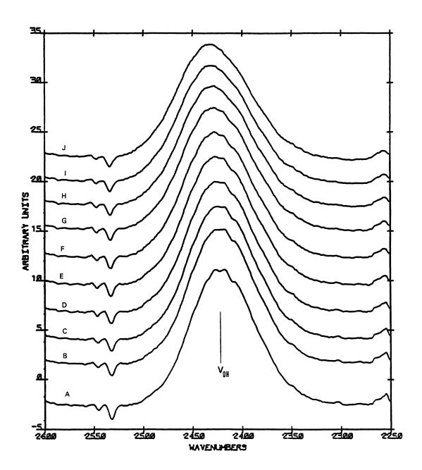
Figure 8. O-D Stretching Absorption of Isolated HOD in the Ethylene Oxide Clathrate Hydrate. A - 110 K; B - 120 K; C - 130 K; D - 140 K; and E - 150 K.
