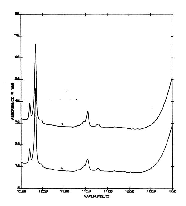
Figure 14. Ethylene Oxide Clathrate Hydrate. A - 80 K and B - 10 K.
