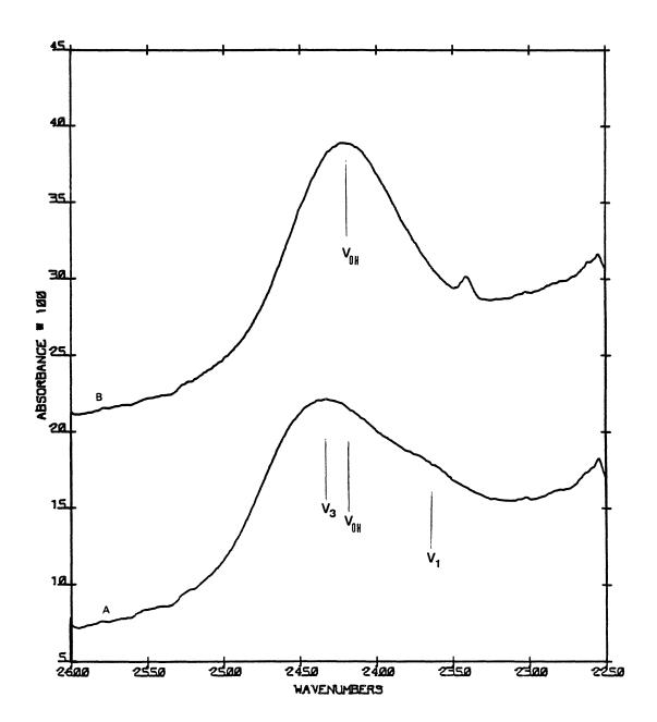
Figure 17. Isolated HOD Subtracted from the After Irradiation of Ethylene Oxide Clathrate Hydrate with 1.7 MeV Electrons.
