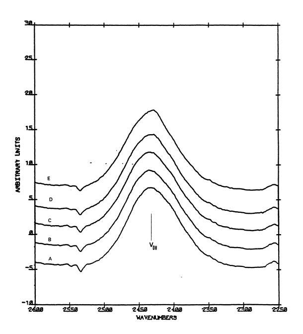
Figure 9. Isolated D<sub>2</sub>O Absorption in the Ethylene Oxide Clathrate Hydrate. A - 10 K; B - 20 K; C - 30 K; D - 40 K; E - 50 K; F - 60 K; G - 70 K; H - 80 K; I - 90 K; and J - 100 K.
