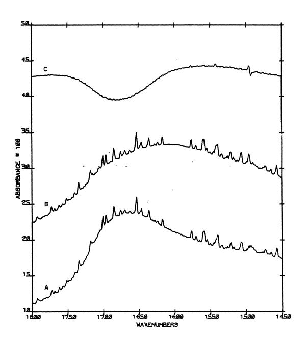
Figure 47. Comparison of the Transition from the Amorphous Mixture to the Clathrate Hydrate with Different Guest Molecules Enclathrated. A - subtraction from the H<sub>2</sub>S clathrate hydrate; B - subtraction from the ethylene oxide clathrate hydrate; and C - subtraction from the SO<sub>2</sub> clathrate hydrate.
