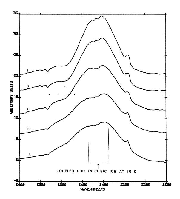
Figure 41. Coupled HOD Generated in Cubic Ice by Irradiation of 1.7 MeV Electrons at 10 K. A - before annealing with 45% of the HOD subtracted and 25% of the D $_2$ O; B - annealed at 140 K with 50% of the HOD subtracted and 20% of the D $_2$ O; C - annealed again at 140 K with 55% of the HOD subtracted and 18% of the D $_2$ O.
