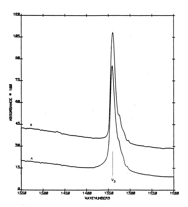
Figure 55. Sulfur Dioxide Enclathrated. A - 140 K; and B - 10 K.
