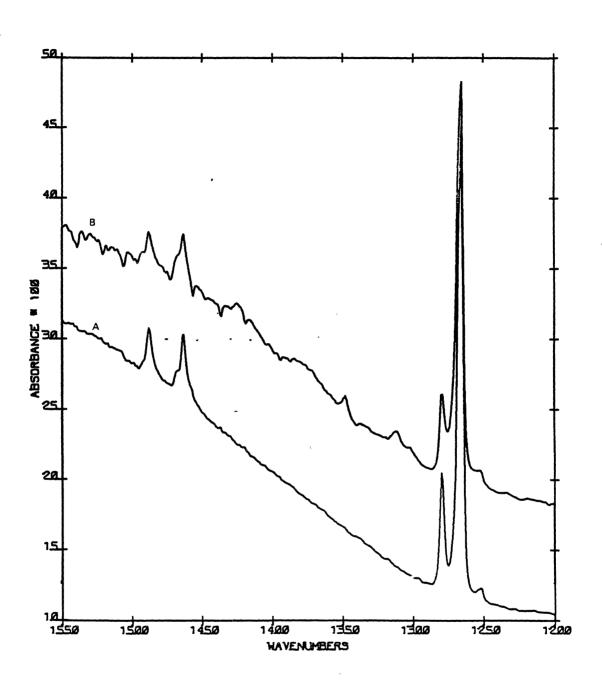
Figure 32. Comparison of the Before (A) and After (B) 1.7 MeV Electron Radiation of the Ethylene Oxide Clathrate Hydrate at 10 K.
