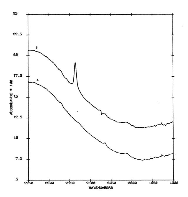
Figure 31. Comparison of the Before (A) and After (B) 1.7 MeV Electron Radiation of the Ethylene Oxide Clathrate Hydrate at 10 K.
