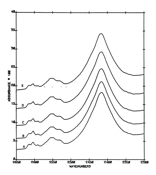
Figure 45. Hydrogen Sulfide Enclathrated. A - 130 K; B - 80 K; C - 50 K; and D - 10 K.
