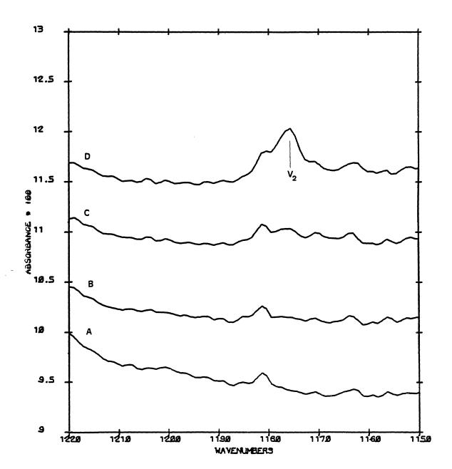
Figure 46. Transition from the Amorphous Mixture of H<sub>2</sub>S and Water to the H<sub>2</sub>S Clathrate Hydrate at 10 K. A - amorphous mixture; B - H<sub>2</sub>S clathrate hydrate; and C - subtraction of the amorphous mixture spectrum from the H<sub>2</sub>S clathrate hydrate spectrum.
