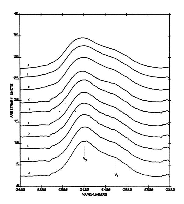
Figure 10. C-H Stretching Absorption of the Ethylene Oxide Molecule in the Clathrate Hydrate. A - 80 K and B - 10 K.
