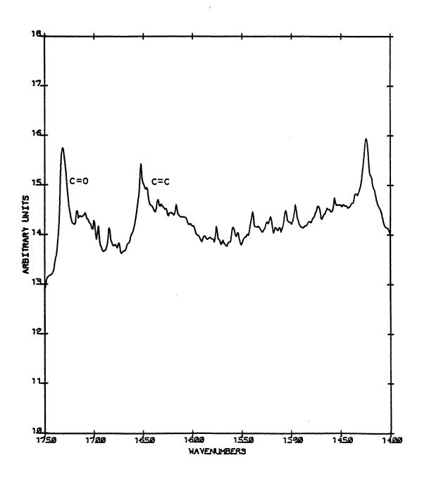
Figure 35. Subtraction of the Before Irradiation Spectrum from the After Irradiation Spectrum.
