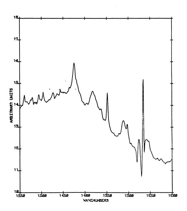
Figure 36. Subtraction of the Before Irradiation Spectrum from the After Irradiation Spectrum.
