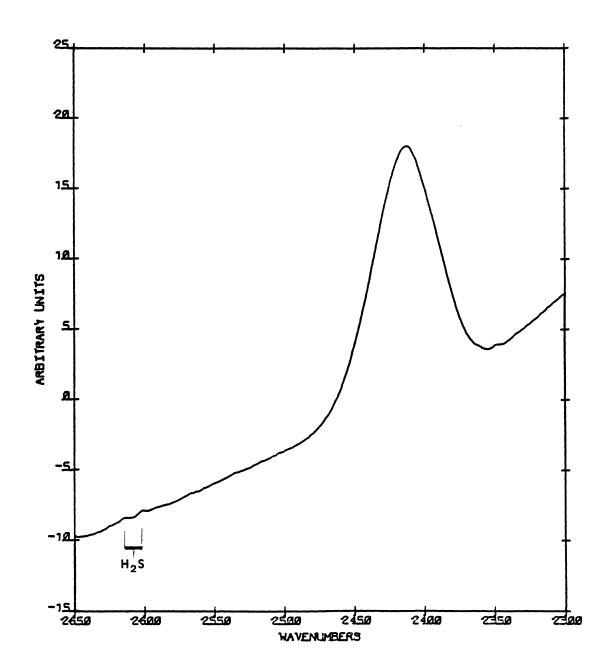
Figure 50. Subtraction of the THF-H $_2$ S Mixed Type II Clathrate Hydrate at 150 K from 10 K. A - spectral region 2650-2580 cm $^{-1}$ ; and B - spectral region 2580-2510 cm $^{-1}$ .
