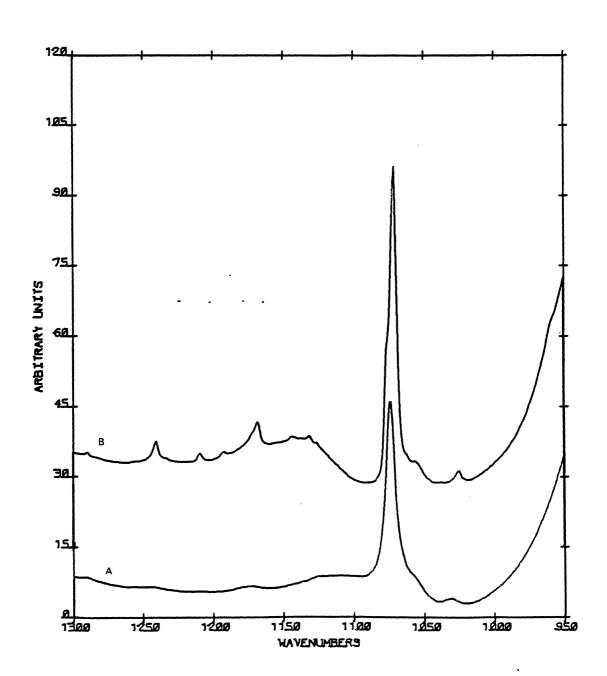
Figure 49. Tetrahydrofuran and  ${\rm H_2S}$  Mixed Type II Clathrate Hydrate at 10 K.
