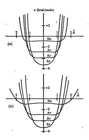
Figure 2. Interaction Energies, ε (kcal/mole) for Guest Molecules in Tetrakaidecahedral Cavities of Type I Hydrates. (a) Variations of E as guest molecule moves through the cage centre along an axis normal to that joining the centres of two opposite hexagonal faces, and parallel to the line joining two opposite water molecules of one of the hexagonal faces. (b) The same as guest moves along the axis of the cavity joining the centres of two opposite hexagonal faces. (Taken from reference 13.)
