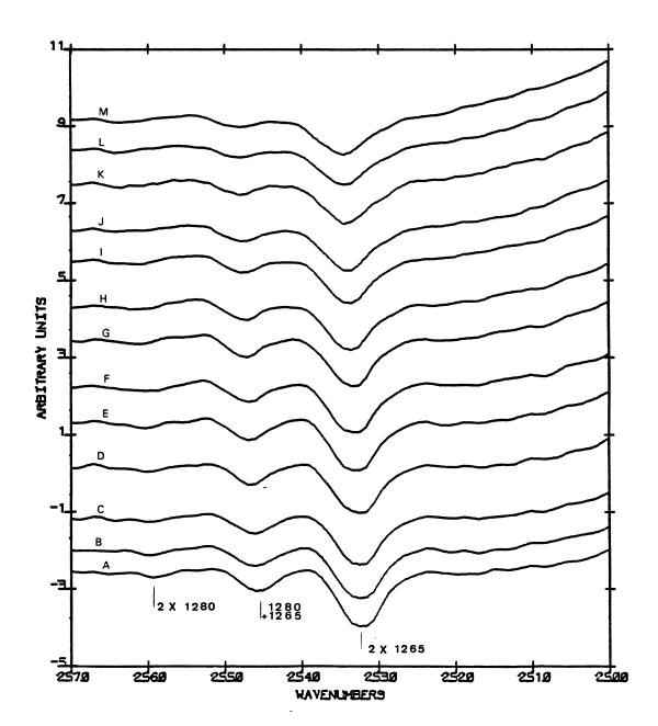
Figure 25. Positive (Non-resonance) Peaks in the Ethylene Oxide Clathrate Hydrate. A - 10 K; B - 20 K; C - 30 K; D - 40 K; E - 50 K; F - 60 K; G - 70 K; H - 80 K; I - 90 K; J - 100 K; K - 110 K; and L - 120 K.
