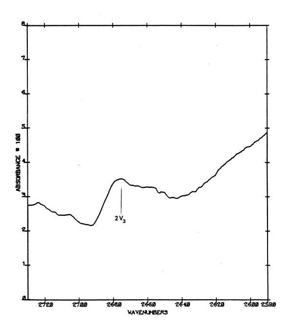
Figure 53. O-D Stretching Absorption Spectrum of the  ${\rm SO}_2$  Clathrate Hydrate at 10 K.
