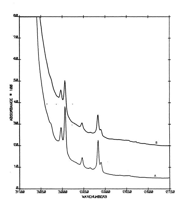
Figure 30. Comparison of the Before (A) and After (B) 1.7 MeV Electron Radiation of the Ethylene Oxide Clathrate Hydrate at 10 K.
