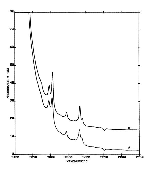
Figure 11. Ethylene Oxide Clathrate Hydrate. A -  $80\ K$  and B -  $10\ K$ .
