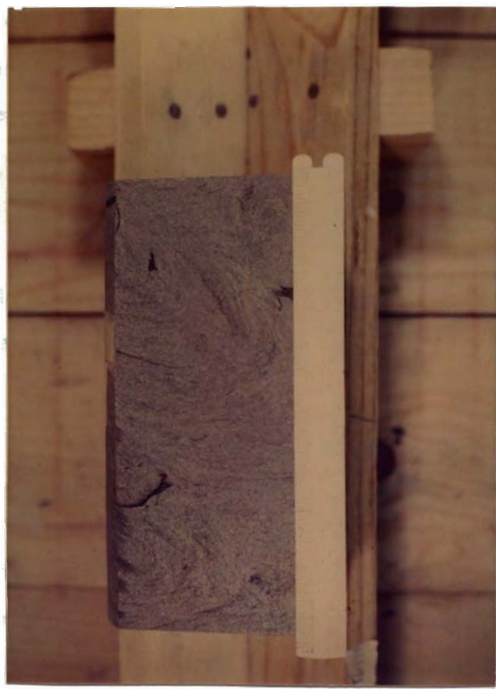
Fig. 20.--Flowage in sandstone, Oklahoma Natural Gas Company Bowling No. 1, depth 10,055 feet.
