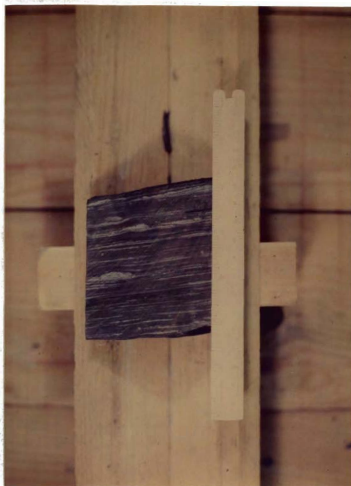
Fig. 18.--Interstratification with dip from Petroleum Inc. Watson No. 1, depth 9896 feet. Note sharp contacts on all beds.
