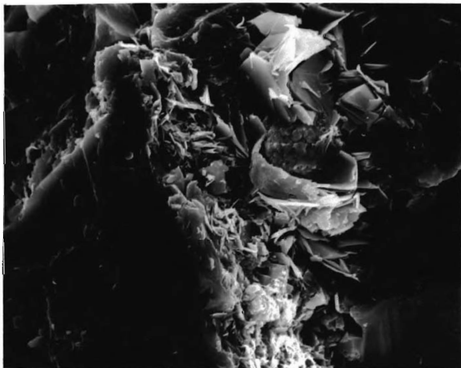
Fig. 28.--Chlorite partially coating corroded quartz grain. Corrosion probably was by earlier-phase carbonate cements (Stage 2 diagenesis) which were subsequently removed by dissolution (Stage 3 diagenesis). Magnification 2000X. Sample from Apexco Inc. Walker No. 1, depth 9912 feet.
