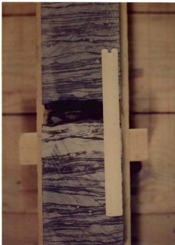
Fig. 17.--Interstratified sandstone and shale from Petroleum Inc. Watson No. 1, depth 9909 feet. Note sharp contacts on all beds.
