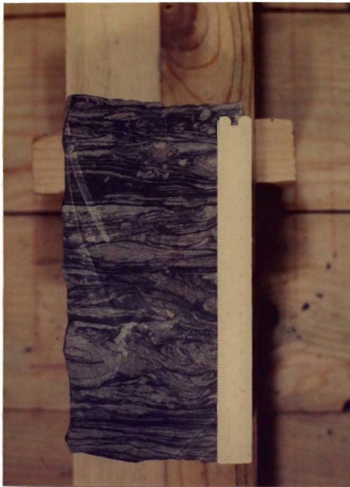
Fig. 19.--Flowage in interstratified sandstone and shale from Amarex No. F-1 Clark, depth 9943 feet.
