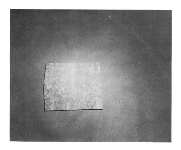
ft./second (.76 m/second) at 20 psi was the most economical for an 800067 nozzle. A nozzle height of 6 in. (15.24 cm) was selected because it was low enough to cover the sample area. Using these constants and a 800067 nozzle it was calculated that each sample area received 0.0047 oz. (0.14 ml) of spray deposit.
