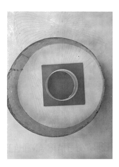
Figure 5. Spray Pattern Showing a Fluorescent Dye on Vinyl Asbestos Tile
