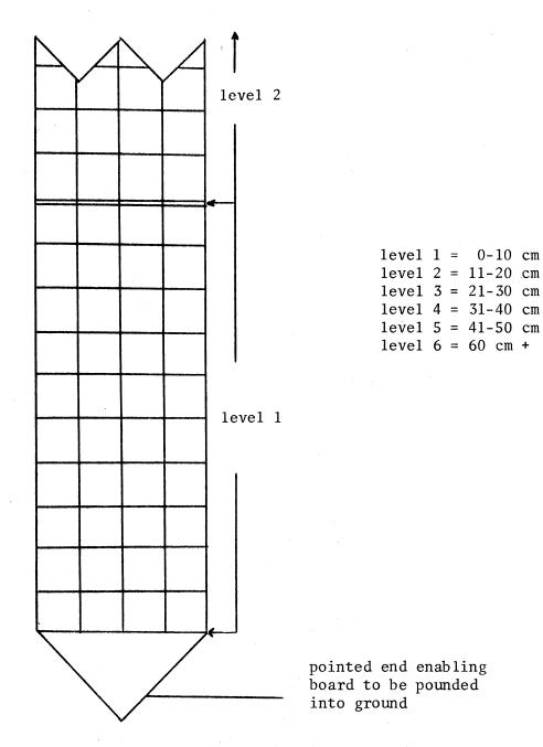
Figure 3. Diagram of density board used to measure aerial vegetation density at singing sites.
