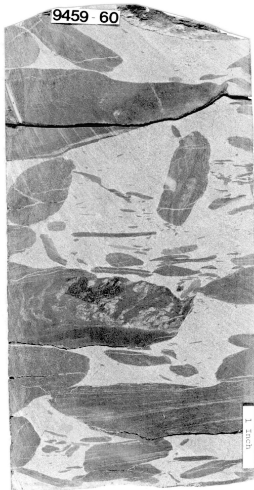
Figure 3. Channel lag features (rip-up clasts) in ARCO, A. M. Kunc No. 3 (Upper Red Fork). Depth, 9459 feet.
