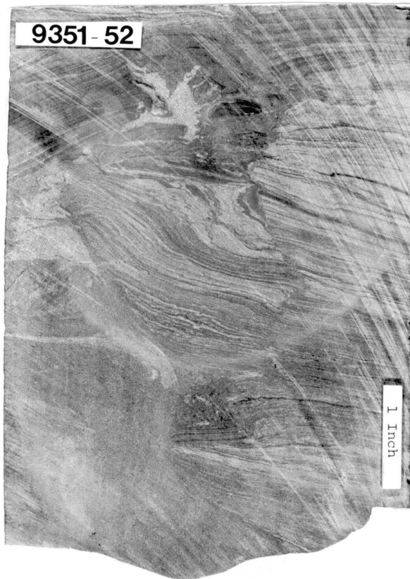
Figure 11. Slump structure, ARCO, Presley No. 2. Depth, 9351 feet (Upper Red Fork).
