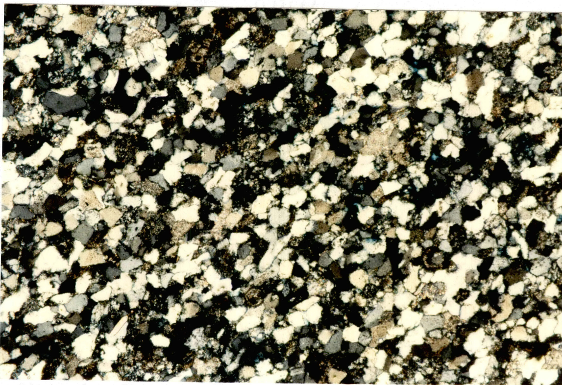
Figure 36. Fine grained quartz grains make up the framework structure in the upper Red Fork sandstone. W. C. P. Leslie No. 1. Depth, 9434 feet (Crossed Nicols) (X40).
