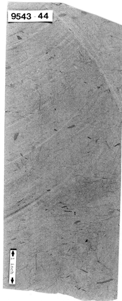
Figure 8. Rippled sandstone (disturbed bed), Wesley Clark No. 2. Depth, 9543 feet (upper Red Fork).
