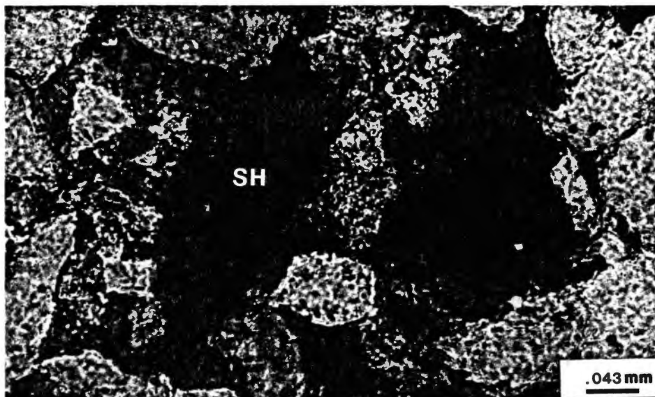
Figure 46. Photomicrograph of Shale Rock Fragments (200X, PPL)
