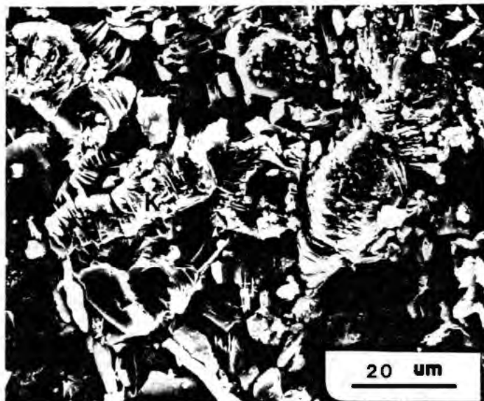
Figure 54. SEM Photomicrograph Illustrating Kaolinite Forming Booklets of Pseudo-hexagonal Crystals (1000X)
