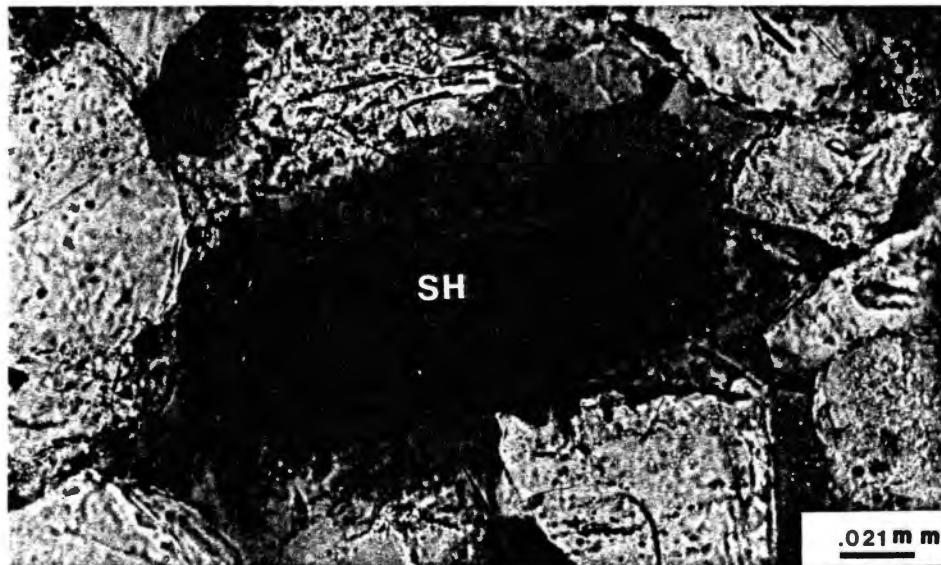
Figure 62. Photomicrograph of A Partially Dissolved Shale Fragment (400X, PPL)
