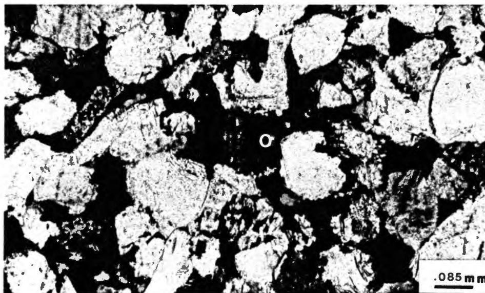
Figure 80. Photomicrograph Illustrating Association of Oil with Secondary Porosity (100X, PPL)
