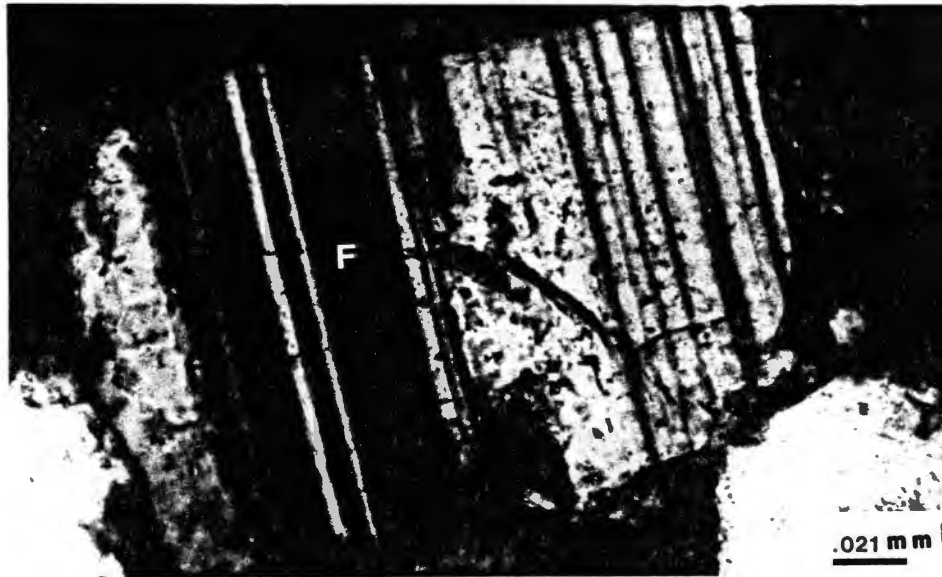
Figure 44. Photomicrograph of Plagioclase Feldspar Grain (400X, XN)
