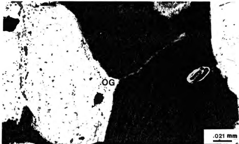
Figure 51. Photomicrograph of Detrital Quartz Grains with Syntaxial Quartz Overgrowths (400X, XN)
