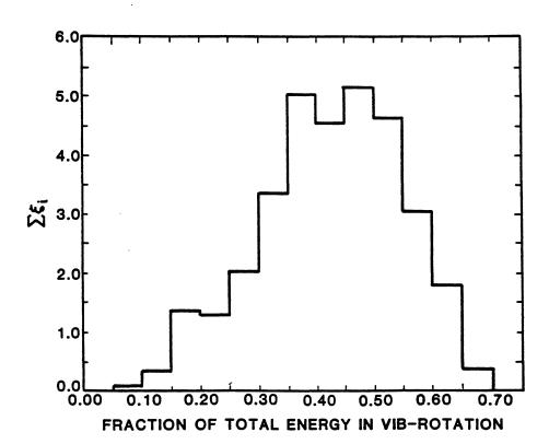
Figure 11. Product Energy Distribution for (D,H) Exchange Reaction on Surface I at  $\rm E_{T}$  = 7.0 kcal/mole.
