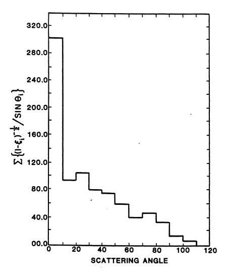
Figure 17. Differential Scattering Cross Section for Br Scattering in (H,H) Abstraction Reaction on Surface III at  $\rm E_T$  = 0.5 kcal/mole.
