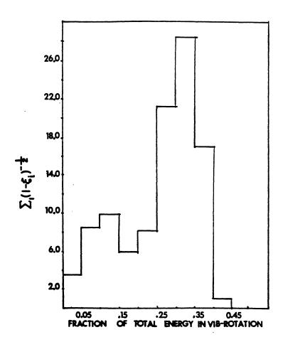
Figure 14. Product Energy Distribution for (H,D) Abstraction Reaction on Surface III at  $\rm E_T$  = 2.0 kcal/mole.
