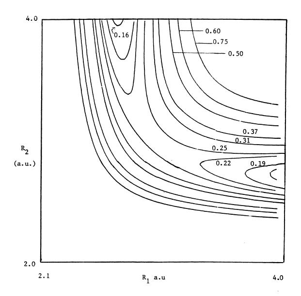
Figure 7. Contour Map for Collinear  $H_{\overline{R_1}}Br_{\overline{R_2}}H$ ,  $\theta$  = 180° on Surface III. Contour values are given in eV on this contour map.
