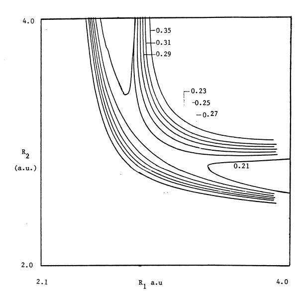
Figure 8. Contour Map for Collinear  $H_{\overline{R_1}}Br_{\overline{R_2}}H$ ,  $\theta$  = 180° on Surface I. Contour values are given in eV on this contour map.
