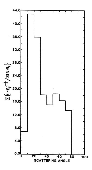
Figure 18. Differential Scattering Cross Section for H Atom Scattering in (D,H) Exchange Reactions on Surface III at  $E_{\rm T}$  = 7.0 kcal/mole.
