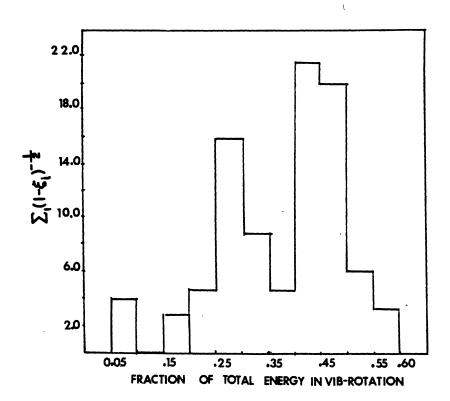
Figure 13. Product Energy Distribution for (H,D) Abstraction Reaction on Surface III at  $\rm E_{T}$  = 0.5 kcal/mole.
