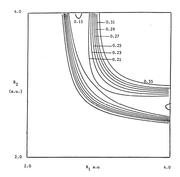
Figure 5. Contour Map for Collinear  $H_{\overline{R_1}}Br_{\overline{R_2}}H$ ,  $\theta$  = 90° on Surface III. Contour values are given in eV on this contour map.
