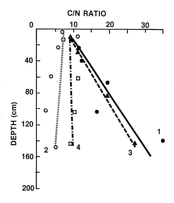
ratios increase to a depth of 160 cm for the relatively old soils of Pit 3, and especially Pit 1, possibly because of the abundance of the resistant forms of organic carbon such as lignins (Kononova, 1966). These ratios are expected to eventually decrease at greater depths than measurable because of the current extremely low levels of organic matter (Speir and Ross, 1982).
