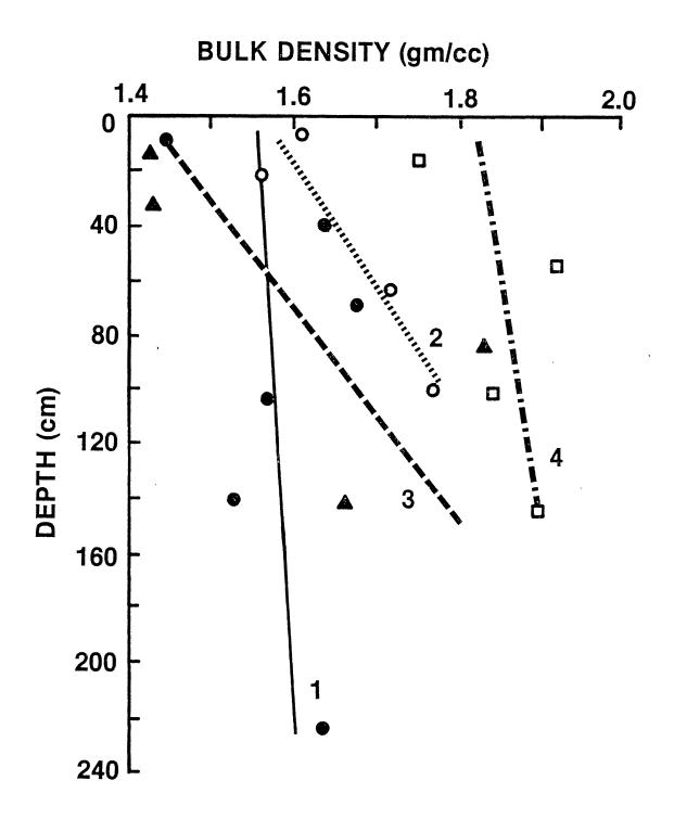
a soil profile. Bulk density results support its use as an indicator of soil depth and soil formation, and therefore, indirectly indicate the influence of erosion on the landscape.
