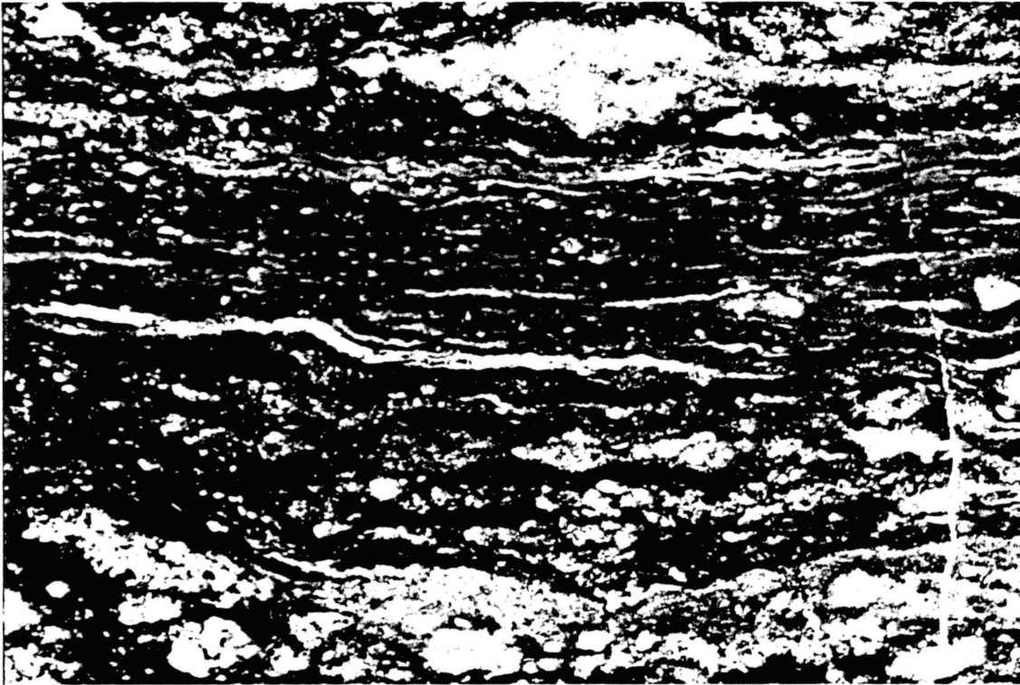
Figure 43. Phosphatic Varves of Cryptocrystalline Carbonate Fluorapatite (X4-PP)
