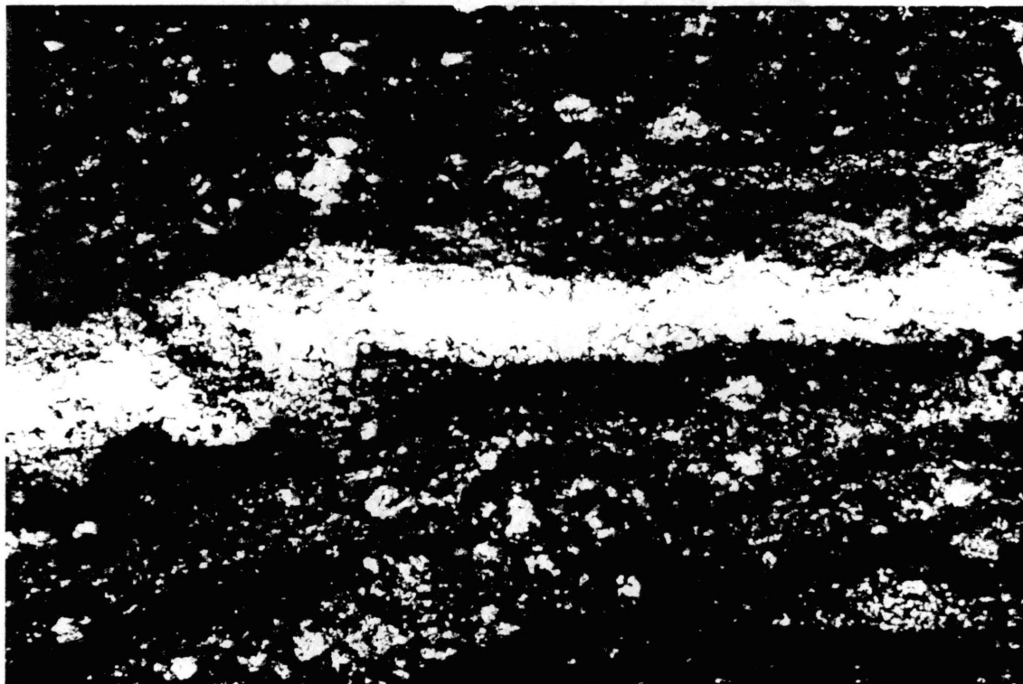
Figure 36. Vein-Filling Chalcedony in the Basinal Deposits (X10-XN)
