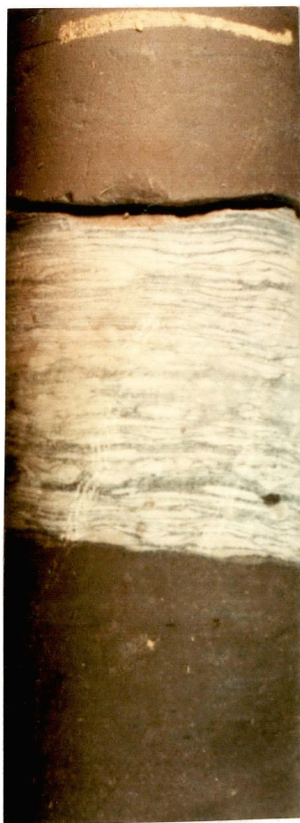
Figure 17. Examples of Thin-Bedded, Interbedded and Interlaminated Siltstones/Shales Characteristic of Portions of the Upper and Lower "Non-Porous" Zones
