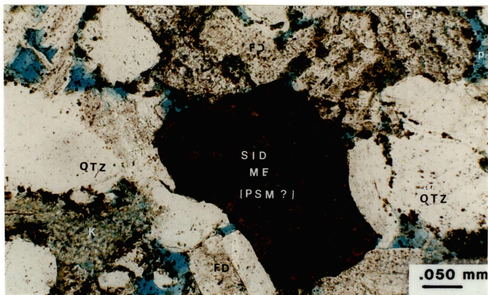
Figure 26. Thin Section Photomicrograph, Plane Polarized Light. Sideritic (SID), Argillaceous Rock Fragment (Mud Fragment) (MF) That Has Undergone Some Ductile Deformation and Can Be Classified Possibly As Pseudomatrix (PSM ?). Kaolinite (K), probably altered clay fragment.
