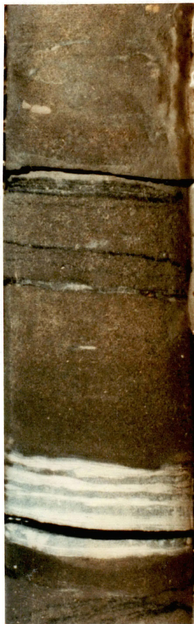
Figure 17. Examples of Thin-Bedded, Interbedded and Interlaminated Siltstones/Shales Characteristic of Portions of the Upper and Lower "Non-Porous" Zones
