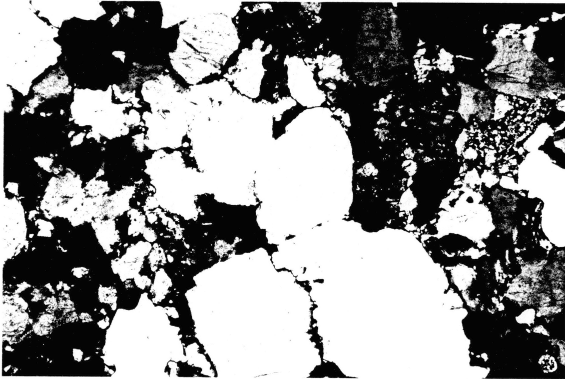
Figure 8. Photomicrograph of Boehm Lamellae from just above the Fractured and Microfaulted Sandstones (100X, XN)
