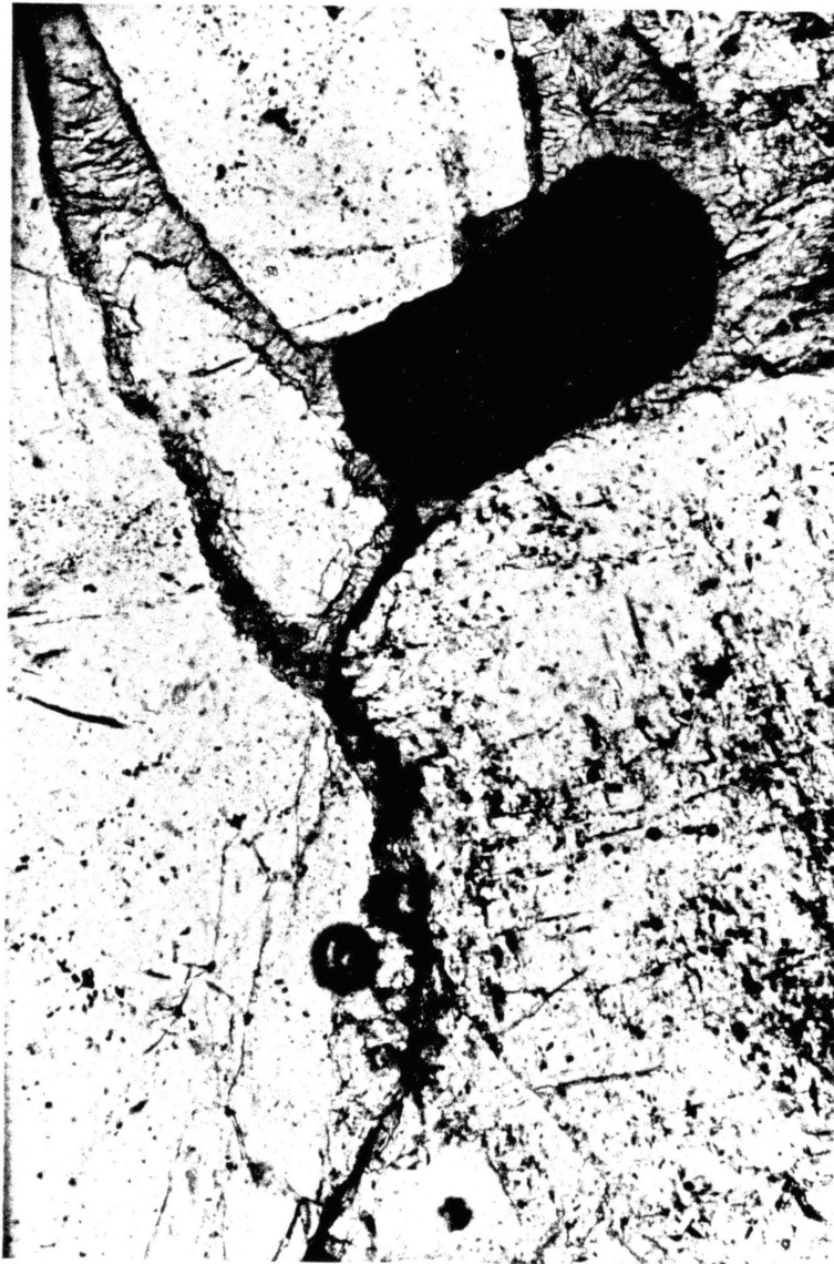
Figure 28. Photomicrograph of Partially Pseudomorphed Biotite Contributing to a Hematite Coating (200X, PPL)
