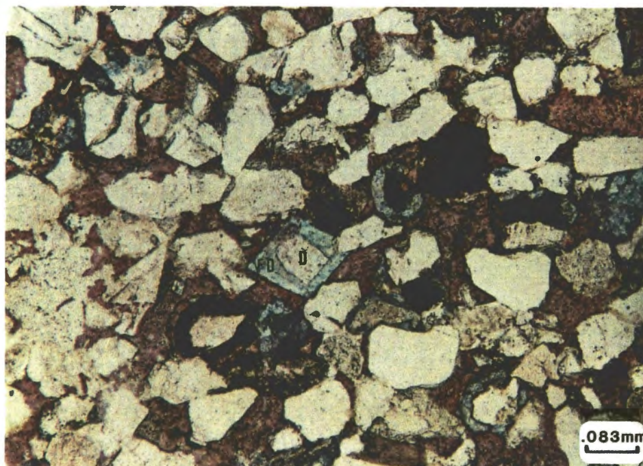
Figure 50. Example of a Euhedral Ferroan Dolomite Crystal (FD), Nucleated on Dolomite (D), and Surrounded by Late Calcite Cement (Stained Red); Also note selective replacement of Ooids by Ferroan Dolomite; Plane Polarized (100X).
