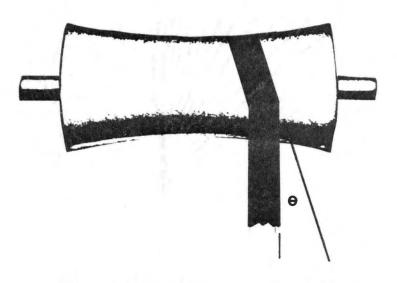
Figure 2. Helix Angle for a Web Strip on a Concave Roll
