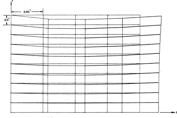
(a) Deformation of the Entry Span
