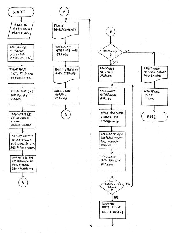
Figure 11. Flowchart for Computer Code CONCAVE.FOR
