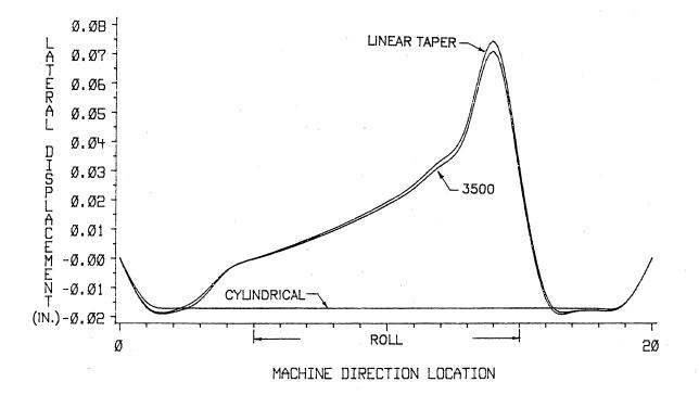
Figure 17. Lateral Displacement of Outside Edge of Web for Circular Arc 3500 and Linear Taper Profiles
