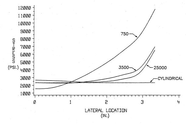
Figure 23. Machine Direction Stresses at Exit of Roll for Circular Arc Profiles
