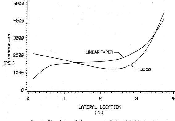
Figure 20. Lateral Stresses at Exit of Roll for Circular Arc 3500 and Linear Taper Profiles
