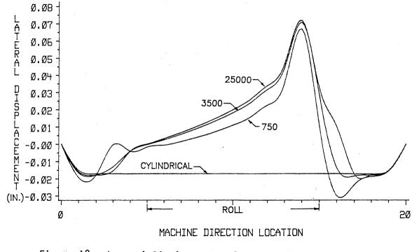
Figure 18. Lateral Displacement of Outside Edge of Web for Circular Arc Profiles
