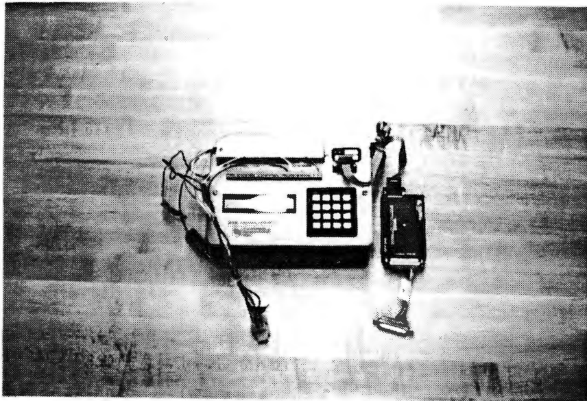
Figure 2. Campbell Scientific model 21X data logger.
