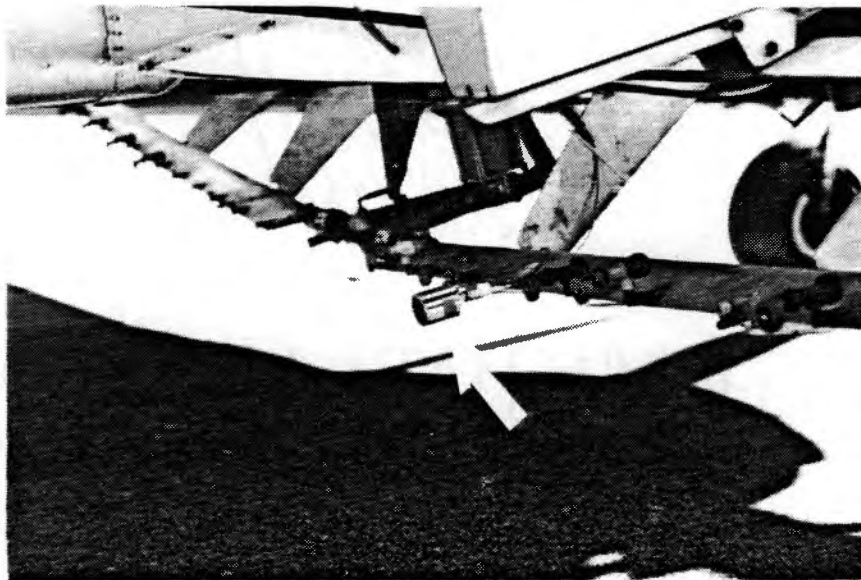
Figure 3. Differential pressure transducer mounted on the spray boom.
