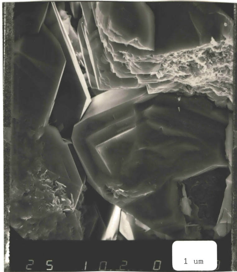
Figure 17. SEM Photomicrograph. Syntaxial quartz overgrowths in a quartzitic sand. Magnification-3000X.
