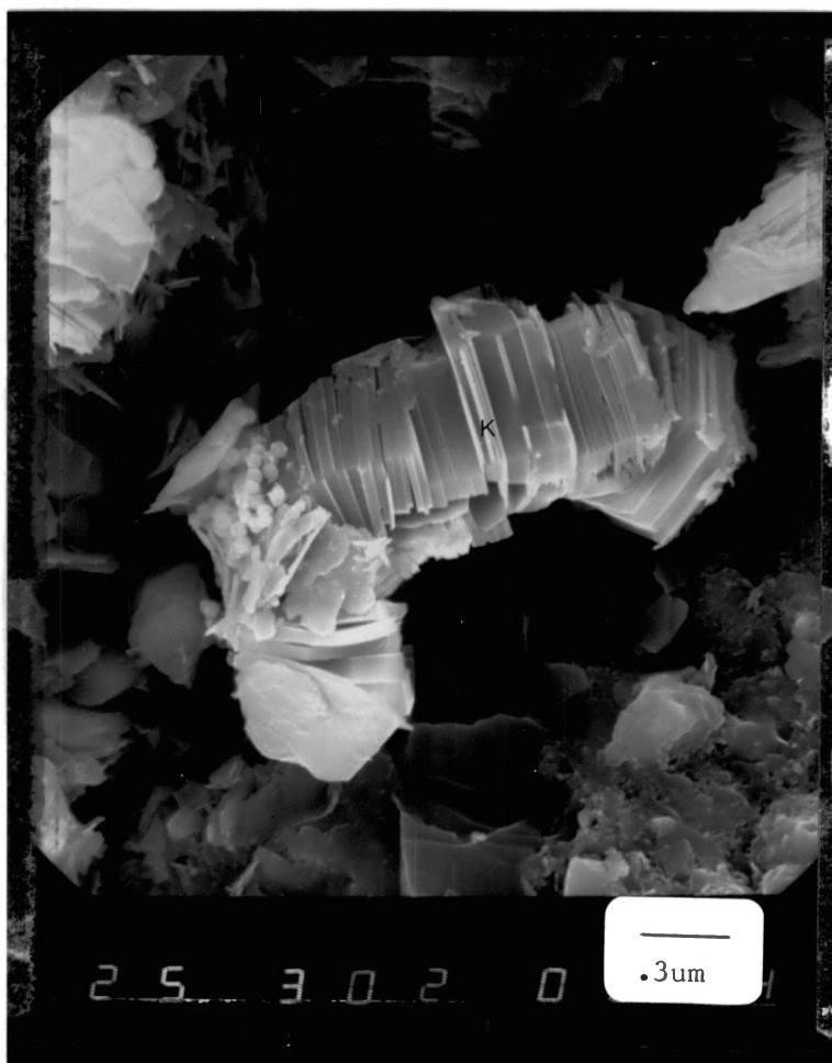
Figure 32. SEM Photomicrograph. Kaolinite (K) filled pores. This authigenic clay had a vermicular morphology and euhedral pseudo-hexagonal crystals. Note authpyrite (arrow) which has precipitated on kaolinite booklets. Magnification - 3000X.
