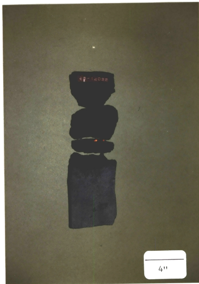
Figure 8. Core from the Apexco, Inc. - Buell No. 1-A demonstrating erosional contact between Lower Britt sandstone and black, laminated, sparsely fossiliferous Cunningham shale.
