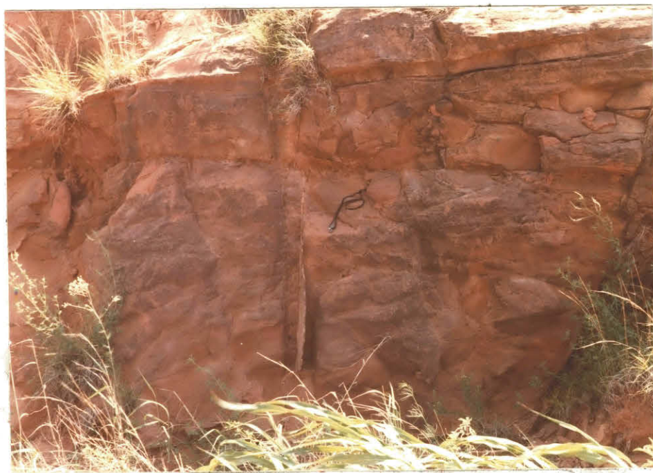
Fig. 10--Jointing found in Elk City Sandstone Sec. 3, T11N R22W.
