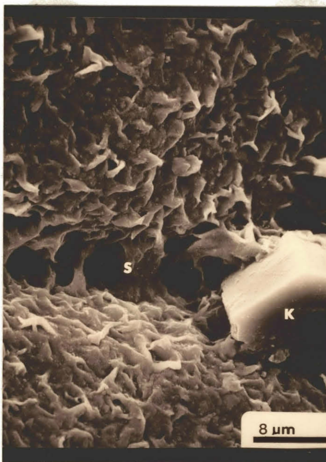
Fig. 19.--SEM photograph of authigenic kaolinite booklets and mixed-layer illite-smectite.
