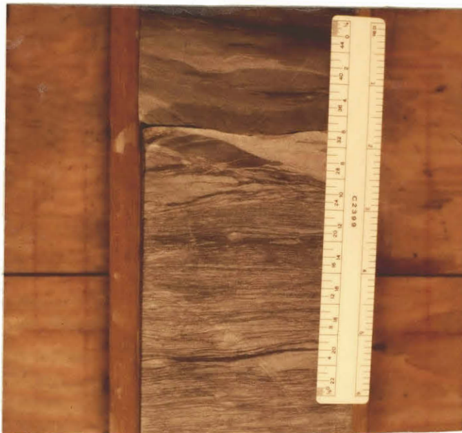
Fig. 17--Sharp contacts between rocks of differing lithology mark an erosional-reactivation surface. From the Getty No. 1 T. R. 16/WSW; depth 4775 ft.
