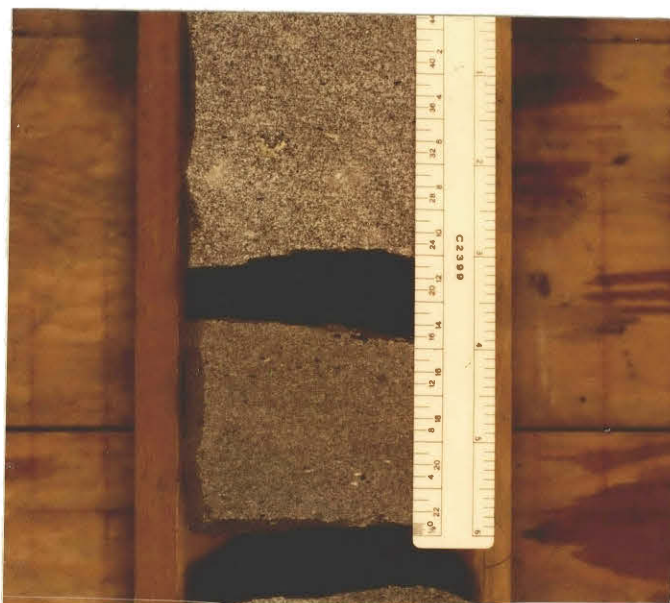
Fig. 14--Horizontally bedded sandstone. From the Texaco C. D. Davis No. 1; depth 4232 ft.
