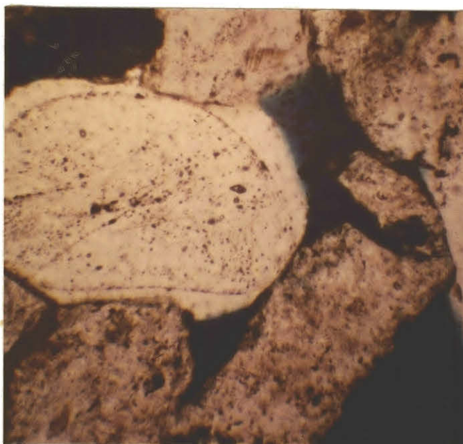
Fig. 34--Extensive development of secondary intergranular porosity is evident by the partial dissolution of quartz overgrowths and corroded nature of the feldspars. Note the dead oil lining and filling many of the pores.
