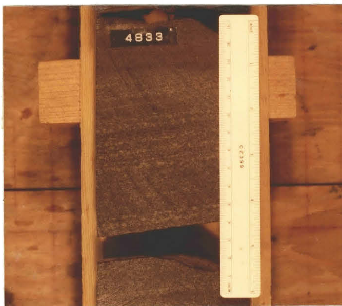
Fig. 13--Horizontally laminated sandstone. From the Getty No. 1 T. R. 16/WSW; depth 4833 ft.
