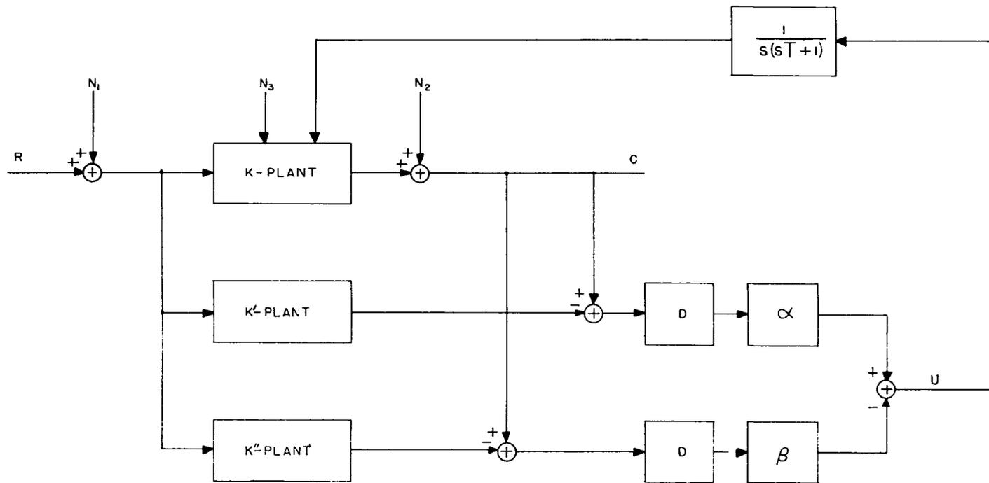
FIG. 20. ERROR FEEDBACK SYSTEM WITH NOISE SOURCES.
