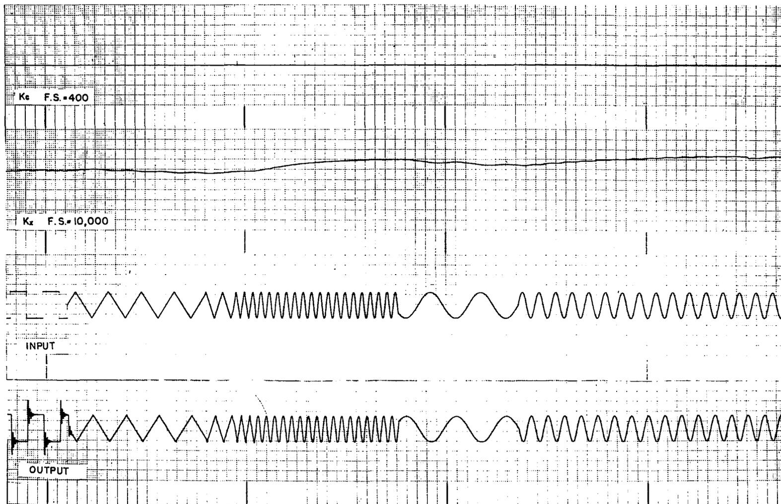
FIG. 26. AIRCRAFT ADAPTIVE PITCH-RATE CONTROL SYSTEM. TIME: 1 SEC./MAJOR DIVISION.
