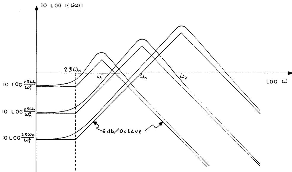
FIG. 3. ENERGY DENSITY FOR DIFFERENT VALUES OF THE PRODUCT  $K_1 K_2$  WHEN THE INPUT IS A STEP. USED BY PERMISSION.
