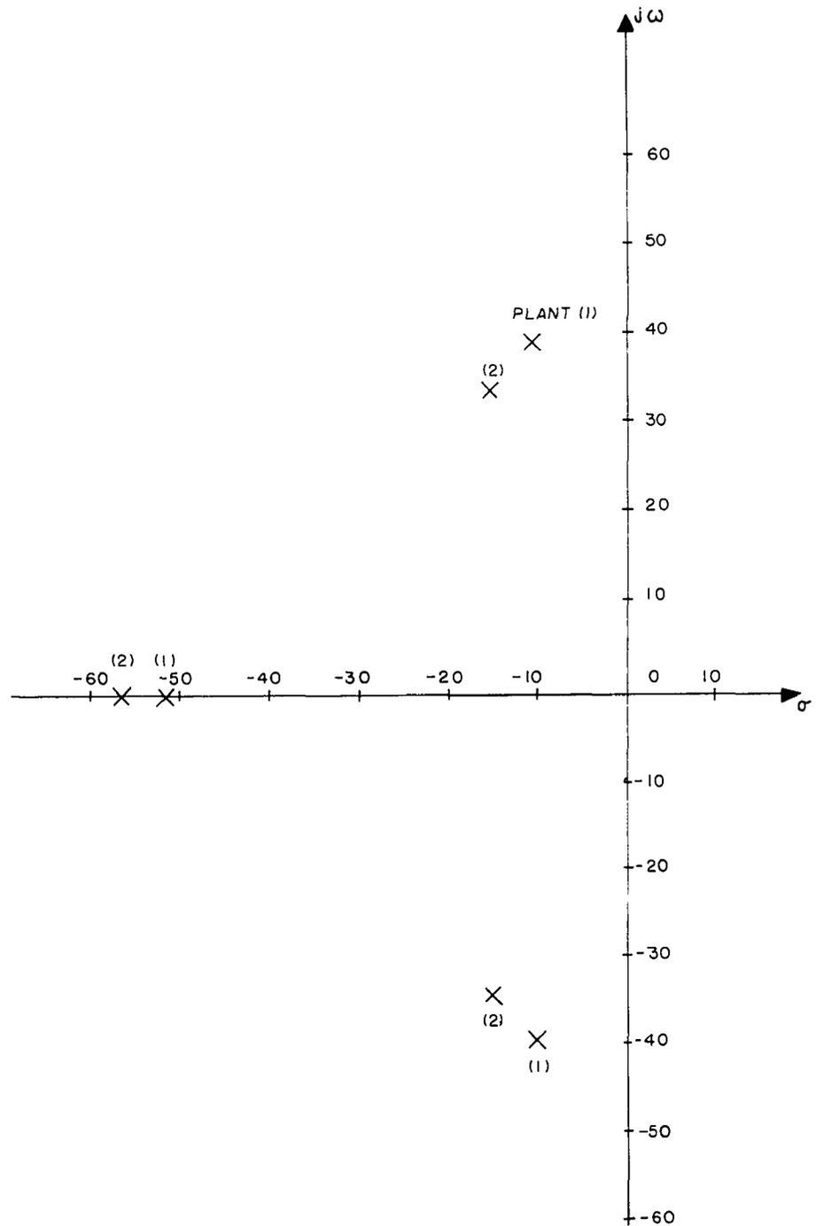
FIG. 27. POSITION OF THIRD-ORDER AUXILIARY PLANT POLES.
