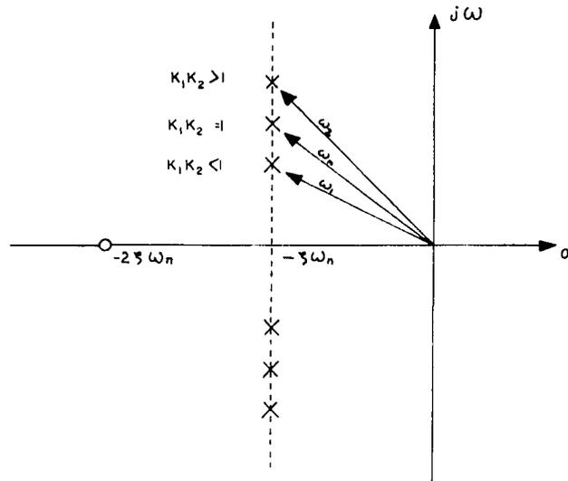
FIG. 2. POLE-ZERO DIAGRAM FOR DIFFERENT VALUES OF THE PRODUCT  $K_1 K_2$  WHEN THE INPUT IS A STEP. USED BY PERMISSION.
