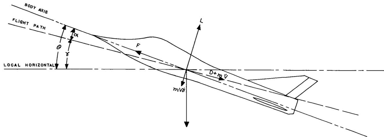
FIG. 21. MOTION OF AN AIRCRAFT WITHIN THE VERTICAL PLANE.
