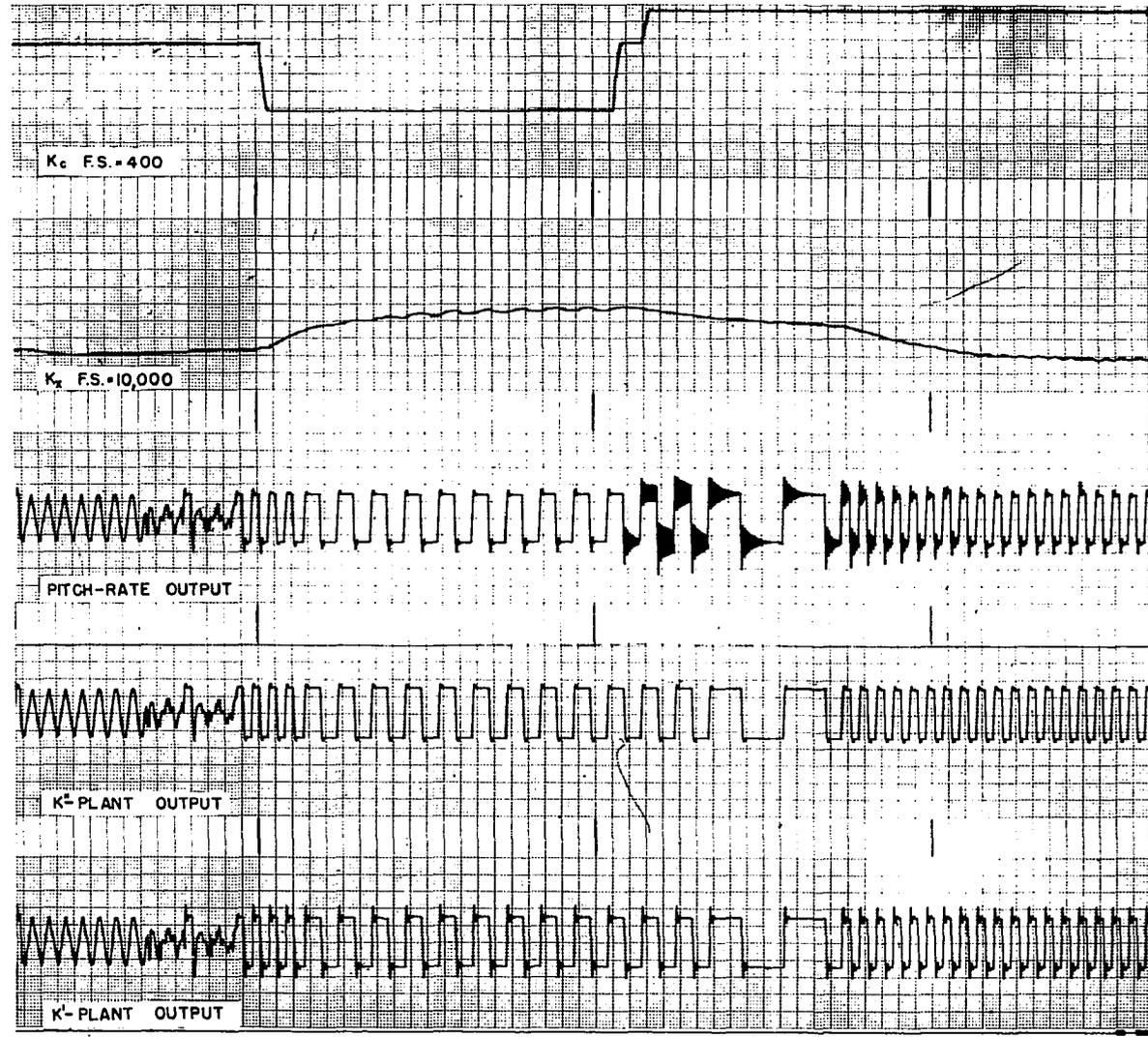
FIG. 30. AIRCRAFT CONTROL SYSTEM AND PLANT OUTPUTS. 1 SEC./MAJOR DIVISION.
