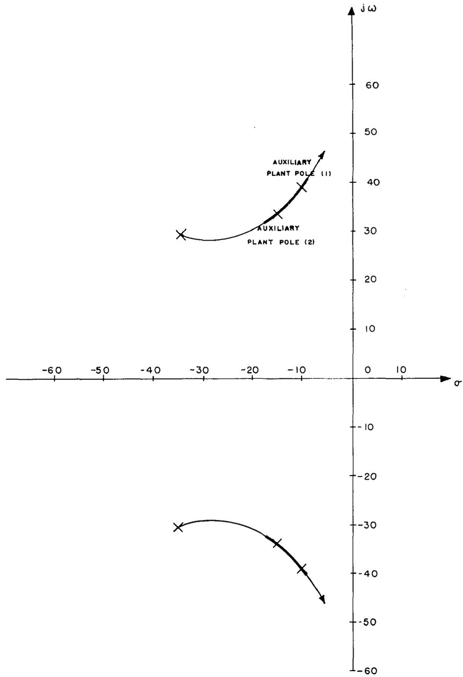
FIG. 24. POSITION OF SECOND-ORDER AUXILIARY PLANT POLES.
