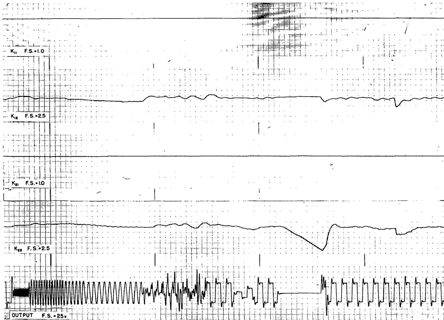
FIG. 37. PARAMETERS OF TWO-PARAMETER ADAPTIVE SYSTEM. TIME: 20 SECONDS = 1 MAJOR DIVISION .
