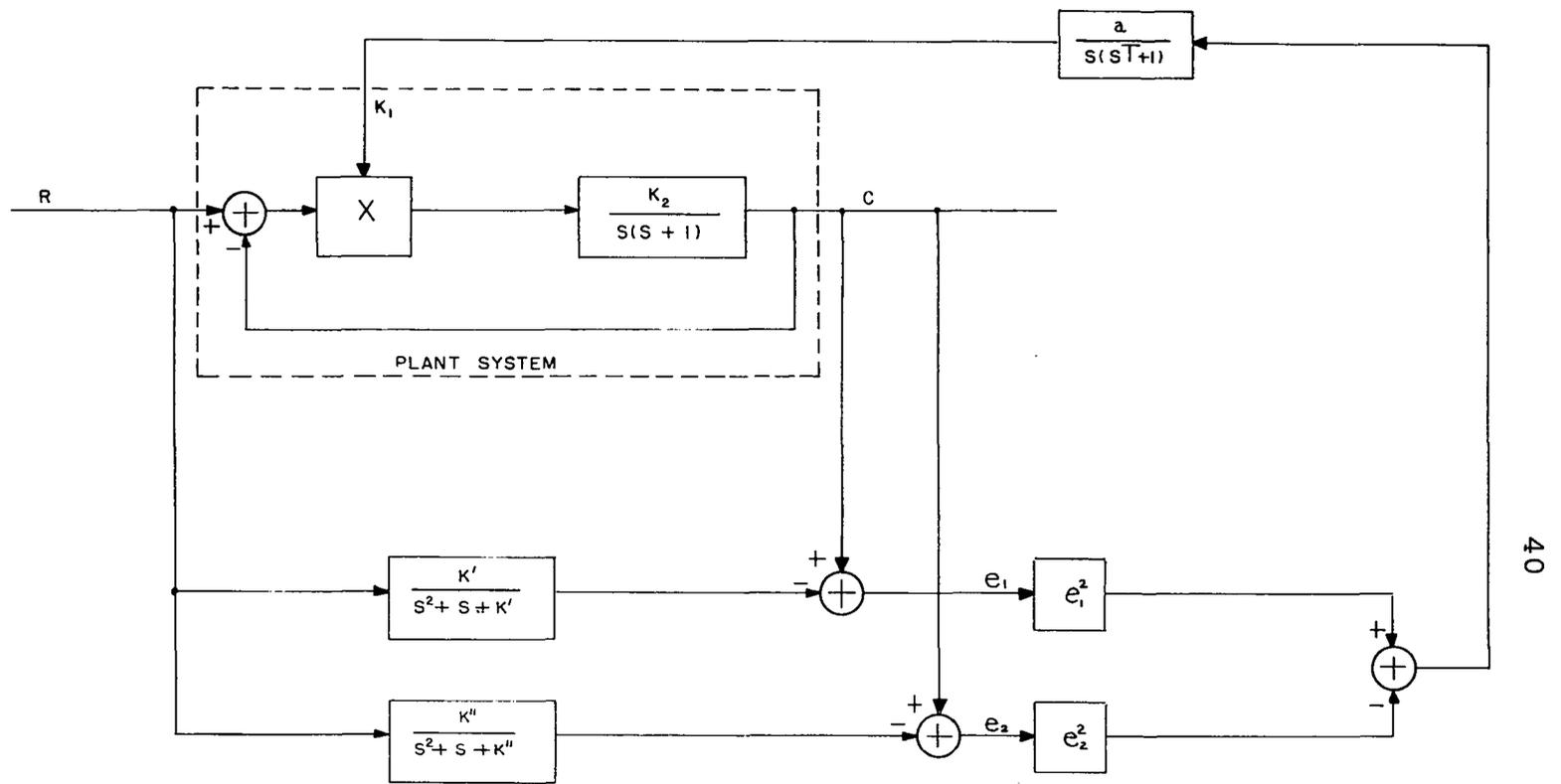
FIG. 12. EXPERIMENTAL SECOND-ORDER PLANT WITH VARIABLE GAIN  $K_2$ .
