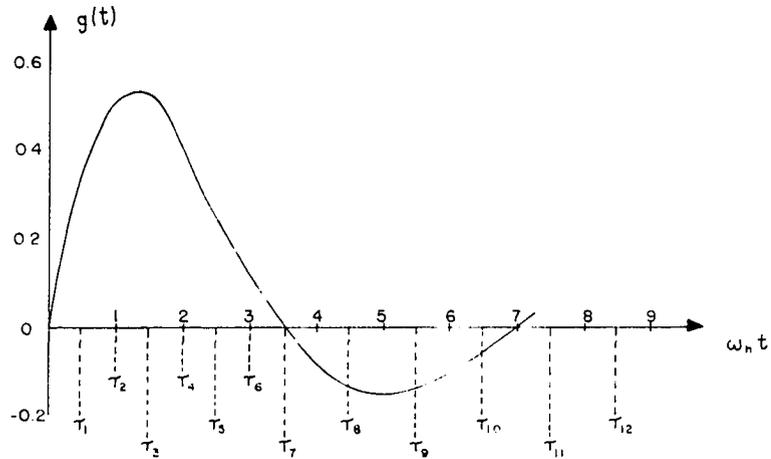
FIG. 8. IMPULSE RESPONSE OF SECOND-ORDER SYSTEM WITH  $\zeta=0.5$ . USED BY PERMISSION.
