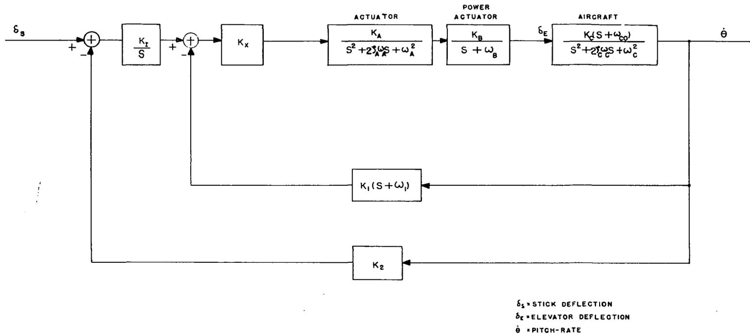
FIG. 22. A PITCH-RATE CONTROL SYSTEM FOR A B-25 AIRCRAFT.
