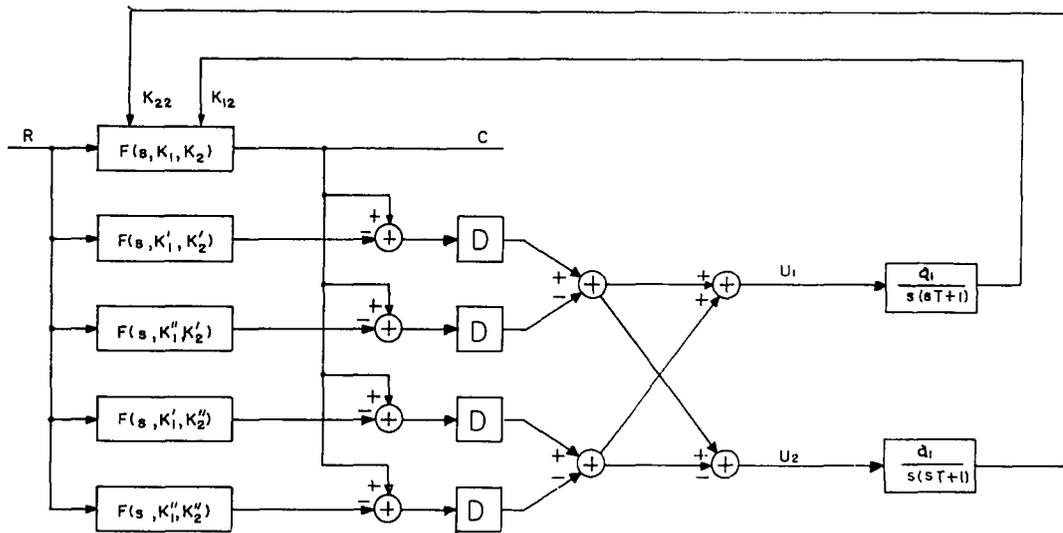
FIG. 33. TWO-PARAMETER ADAPTIVE SYSTEM.
