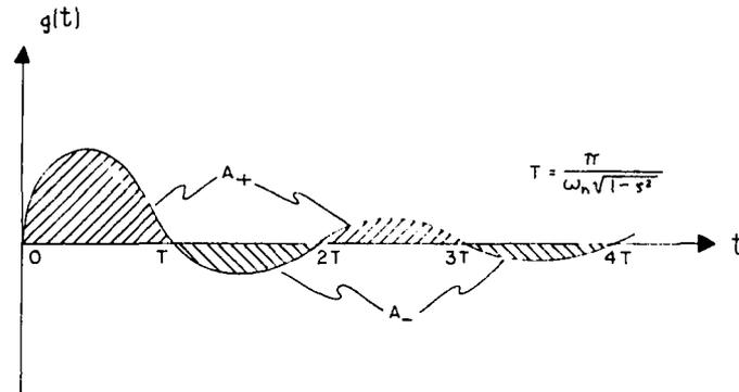
FIG. 6. IMPULSE RESPONSE OF A SECOND-ORDER SYSTEM. FROM ADAPTIVE CONTROL SYSTEMS, BY MISHKIN & BRAUN. COPYRIGHT 1961. MCGRAW-HILL BOOK CO., INC. USED BY PERMISSION.
