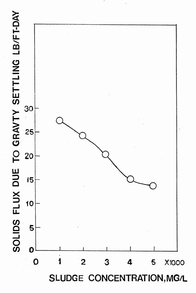
Figure 23. Solids Flux vs. Sludge Concentration at Sludge Age of 6 Days
