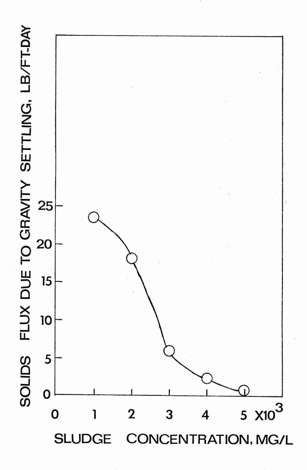
Figure 25. Solids Flux vs. Sludge Concentration at Sludge Age of 10 Days
