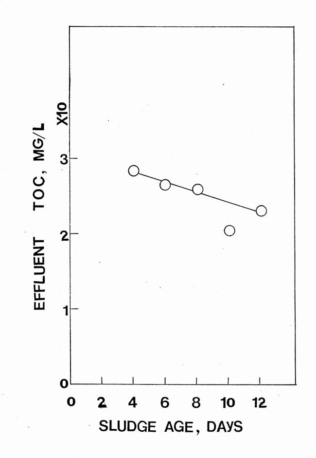
It is seen that high removal efficiencies of BOD and TOC were achieved by the activated sludge unit.
