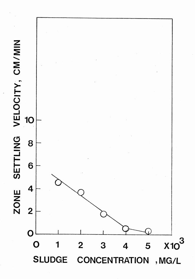
Figure 12. Zone Settling Velocity vs. Sludge Concentration at Sludge Age of 12 Days
