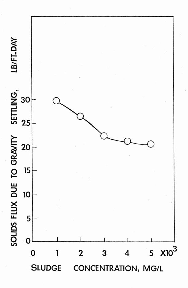
Figure 24. Solids Flux vs. Sludge Concentration at Sludge Age of 8 Days
