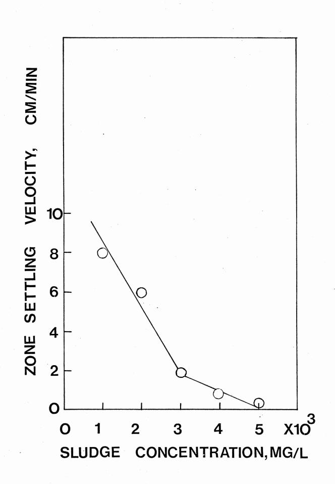
Figure 11. Zone Settling Velocity vs. Sludge Concentration at Sludge Age of 10 Days
