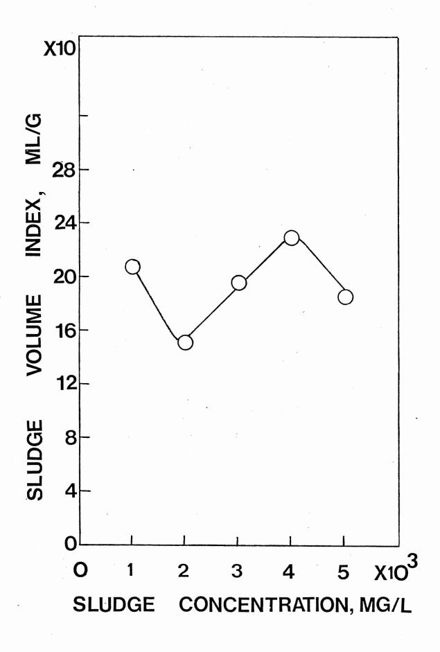
Figure 20. Sludge Volume Index vs. Initial Sludge Concentration at All Studied Sludge Ages
