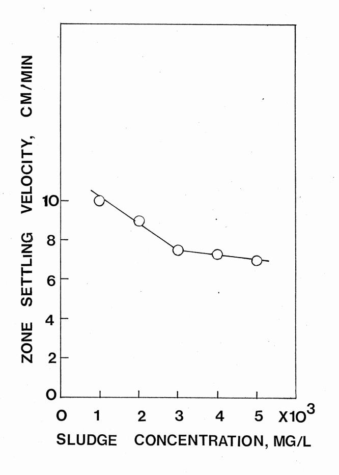
Figure 10. Zone Settling Velocity vs. Sludge Concentration at Sludge Age of 8 Days
