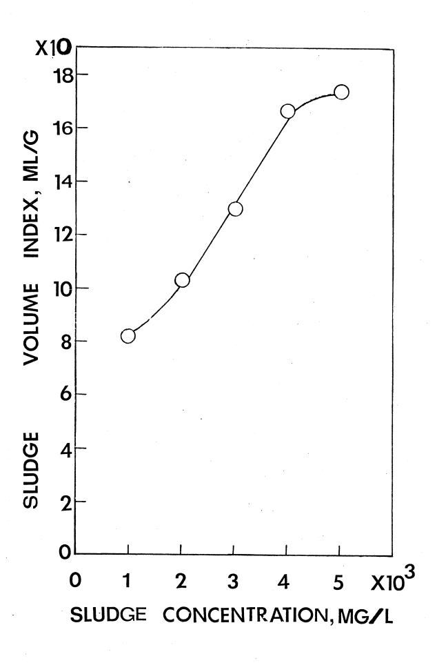
Figure 19. Sludge Volume Index vs. Initial Sludge Concentration at Sludge Age of 12 Days
