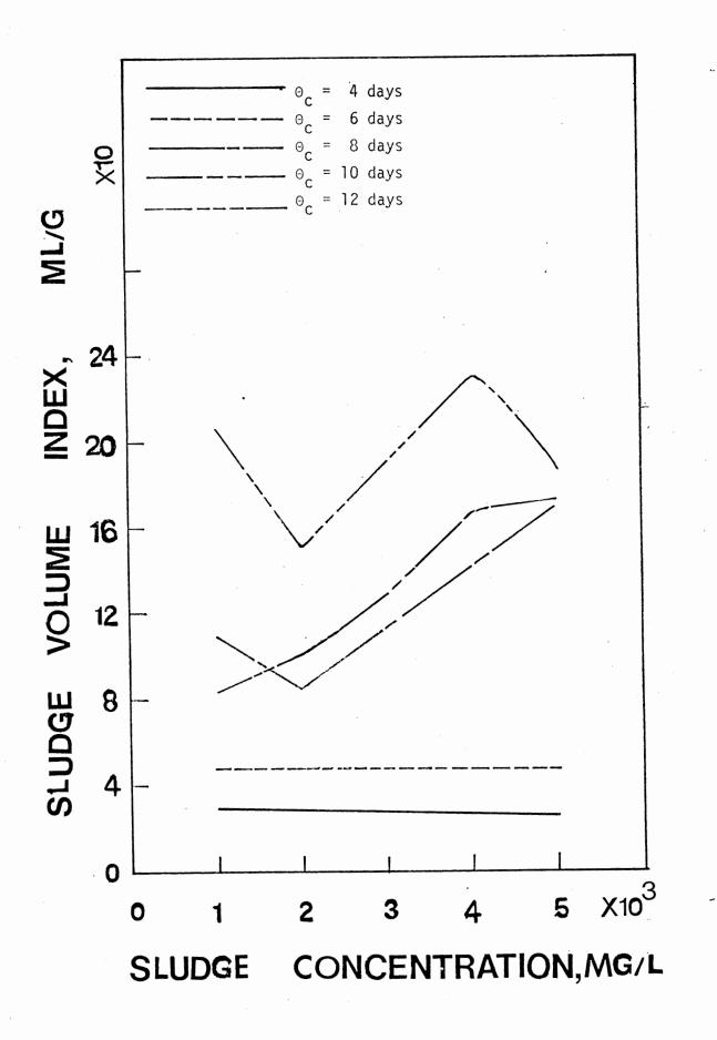
Figure 21. Sludge Volume Index vs. Sludge Age at Various Initial Concentrations
