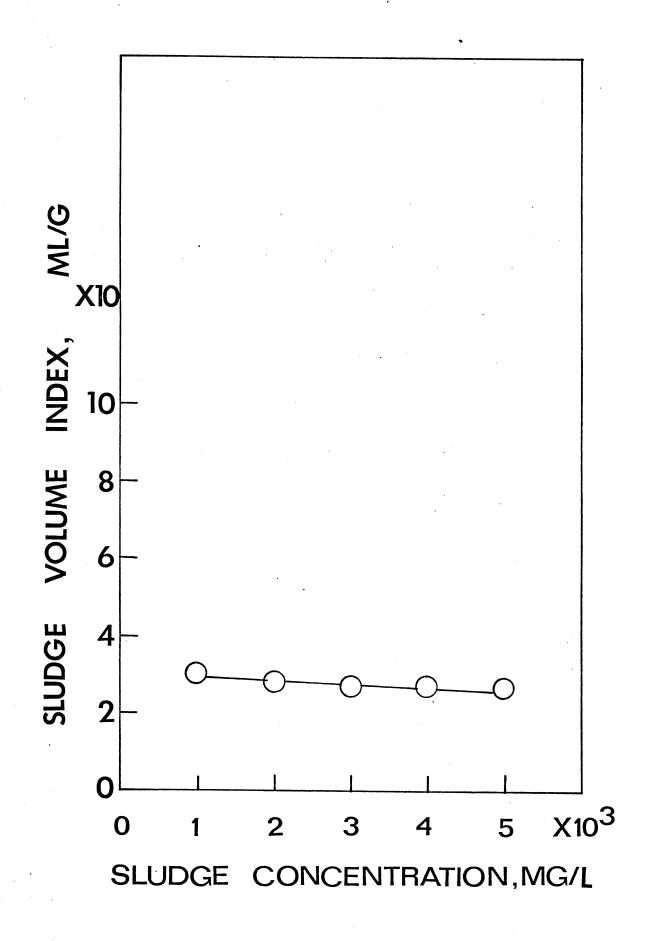
Figure 16. Sludge Volume Index vs. Initial Sludge Concentration at Sludge Age of 6 Days
