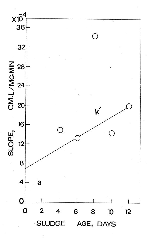
K = slope of the straight line when  $V_0$  is plotted versus  $\Theta_c$ b = the intercept of the above line with vertical axis  $\Theta_c$  = sludge age, day
