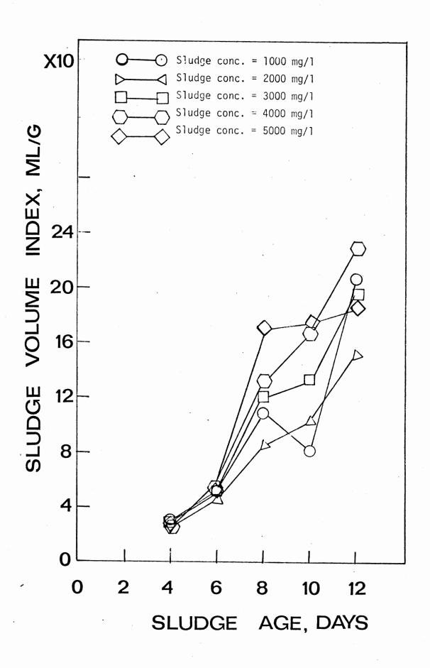
shows a clearer relationship between the sludge volume index and sludge age. From the above figures it can be seen that the 12 day sludge age has the greatest sludge volume index. In other words, the sludge volume index is going to increase from 4-day to 12-day sludge ages. As seen in Chapter II, increasing sludge volume index will result in lower settleability of sludge. In other words, with higher sludge volume index, the zone settling velocity will decrease.
