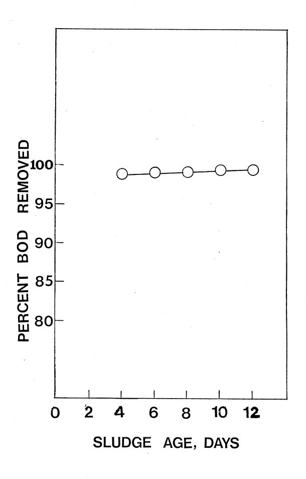
Figure 3. Soluble Effluent BOD vs. Sludge Age
