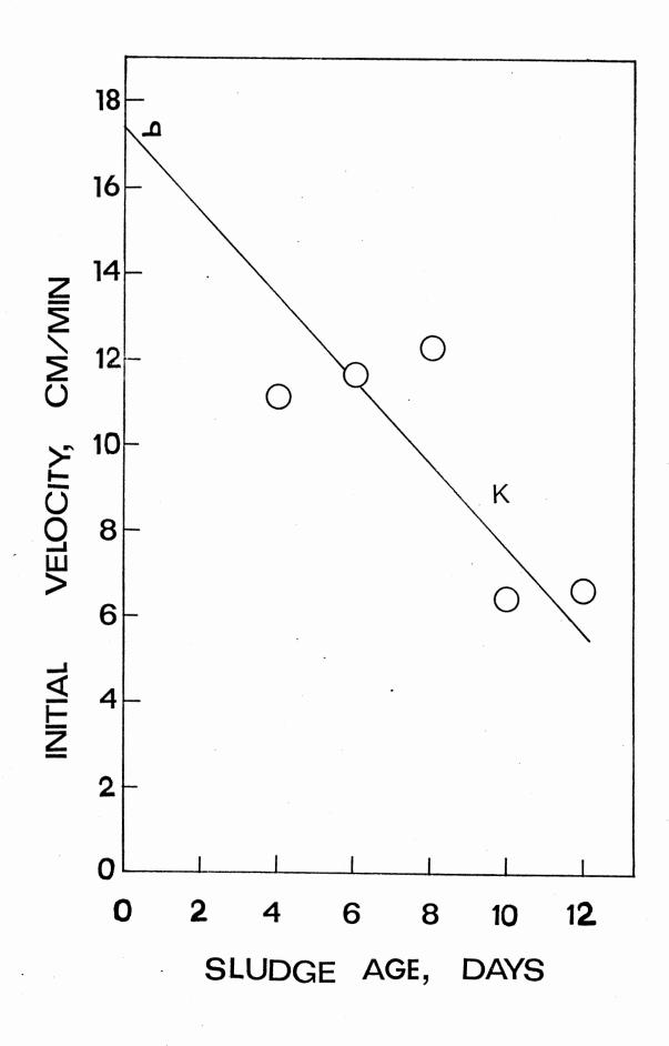
Figure 29. Slope (from Figure 13) vs. Sludge Age
