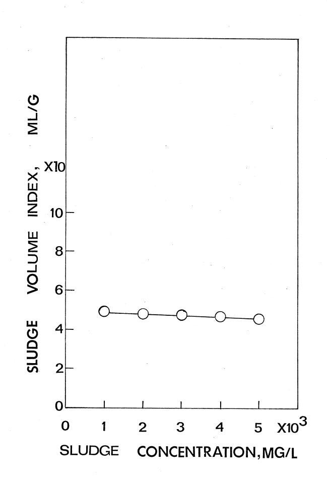
Figure 17. Sludge Volume Index vs. Initial Sludge Concentration at Sludge Age of 8 Days
