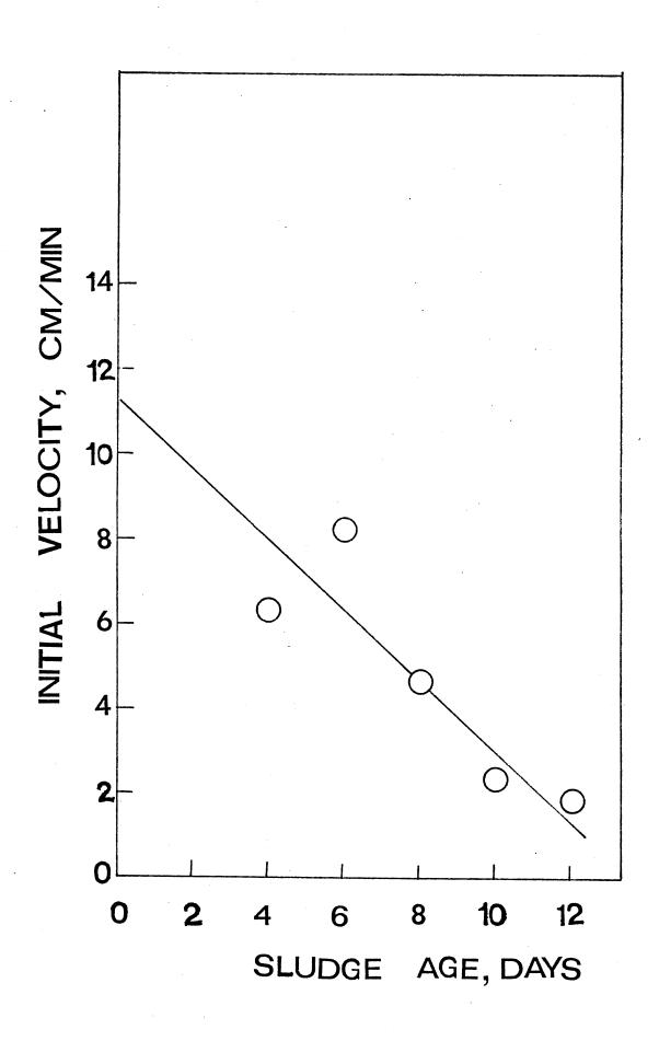
Figure 31. Slope (from Figure 13) vs. Sludge Age
