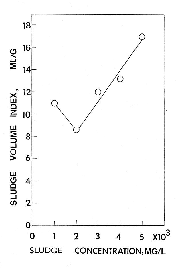
Figure 18. Sludge Volume Index vs. Initial Sludge Concentration at Sludge Age of 10 Days
