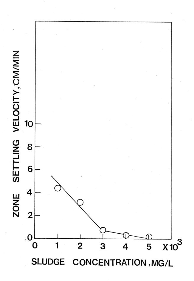
Figure 13. Zone Settling Velocity vs. Sludge Concentration at All Sludge Ages
