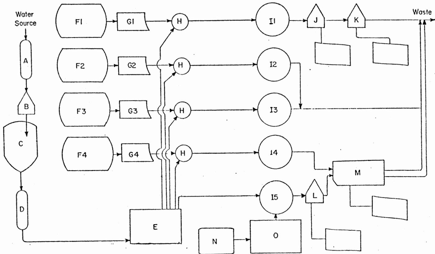
Figure 3. Diluter System Design and Layout. A. Chlorine filter. B. Automatic filler. C. Reservoir. D. Organic removal filter. E. Masterflex Pump. F. Toxicant bottles. G. FMI pumps. H. Mixing Chambers. I. Exposure Chambers. J. Dissolved Oxygen Monitor. K. pH Monitor. L. Temperature Monitor. M. ISCO Concentration Monitor (Spectrophotometer). N. Ethanol Source. O. Ethanol pump. Exposure Chamber Number 5 is used as the control. Arrows denote fluid flow through system.
