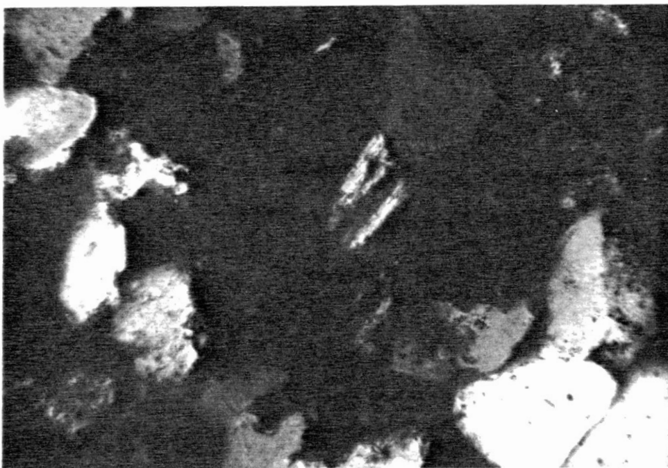
Figure 26. Partially Dissolved Feldspar Grain (Center) Forming Secondary Porosity. Note the Dissolution Along Cleavage, Magnification 100X. (a) Plane-Polarized Light. (b) Crossed-Nicols. Sample From Honolulu Oil Maben No. 2, Depth 6145 Ft.
