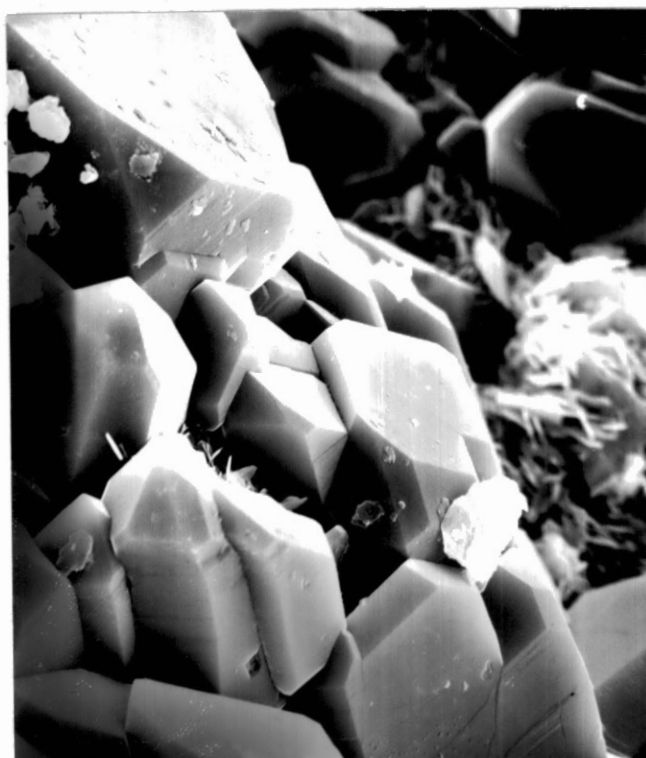
Fig. 45--Scanning electron photomicrograph of euhedral quartz terminations. Magnification 2000X, SEM, Rhodd #1, Depth 4257.6'.
