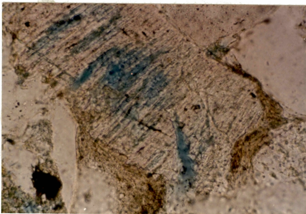
Fig. 42--Photomicrograph of partially dissolved detrital feldspar grain. Magnification 40X, Plane Polarized Light, Coe Bailey #1, Depth 4263.0'.
