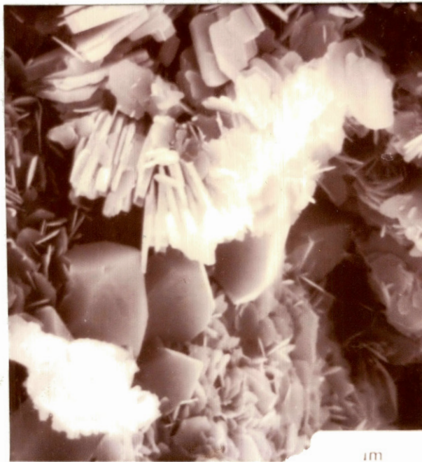
Fig. 50--Scanning electron photomicrograph of authigenic kaolinite. Magnification 1800X, SEM, Coe Bailey #1, Depth 4219.4'.
