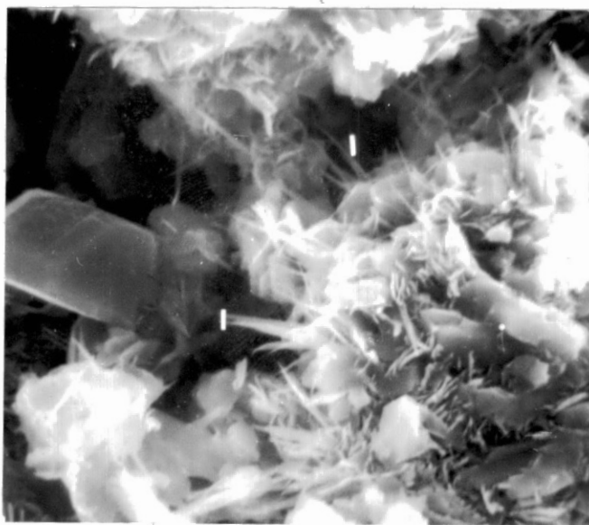
Fig. 31-- Scanning electron photomicrograph of authigenic illite. Magnification 2400X, SEM, Coe Bailey #1, Depth 4263.0'.
