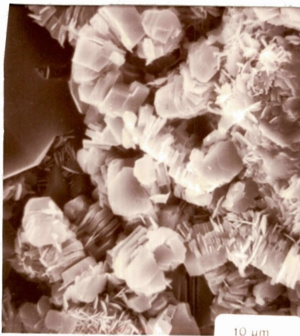
Fig. 29--Scanning electron photomicrograph of authigenic kaolinite. Magnification 2000X, SEM, Coe Bailey #1, Depth 4223.2'.
