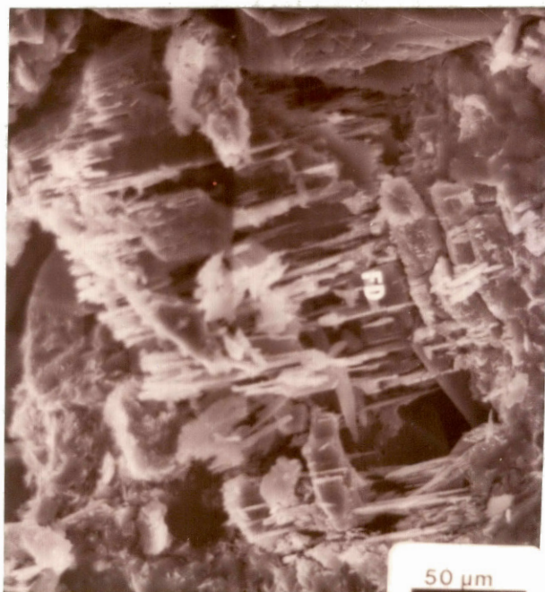
Fig. 44--Scanning electron photomicrograph of a partially leached feldspar grain. Magnification 1600X, Coe Bailey #1, SEM, Depth 4223.2'.
