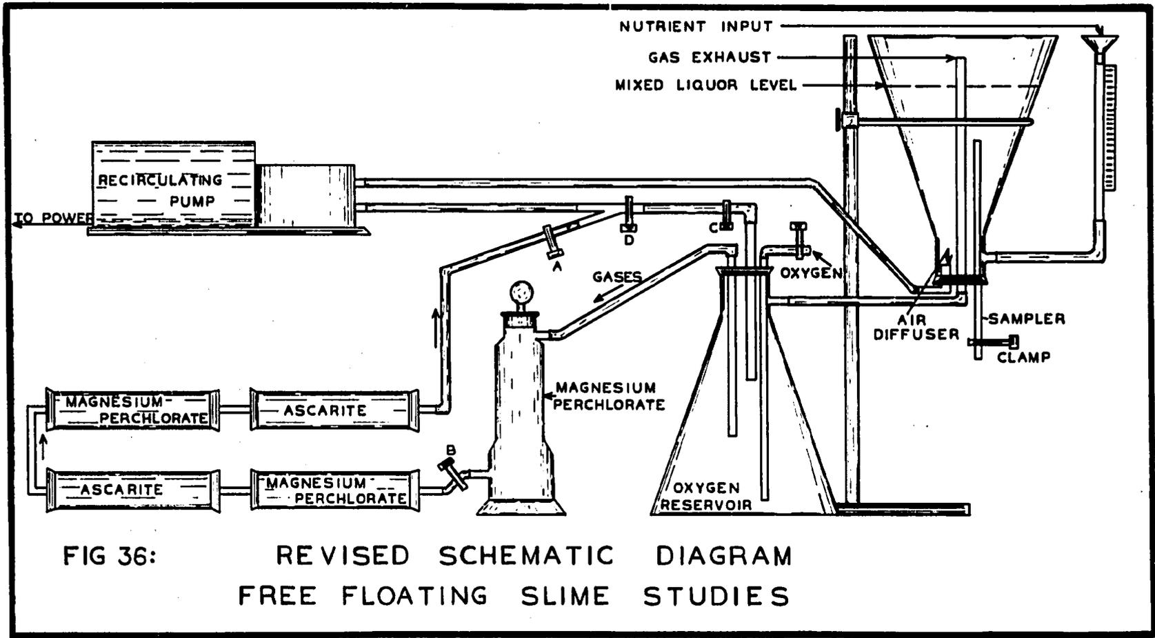
injecting pure oxygen by means of hypodermic syringe. Another tube was connected to a magnesium perchlorate tower leading to an Ascarite train.
