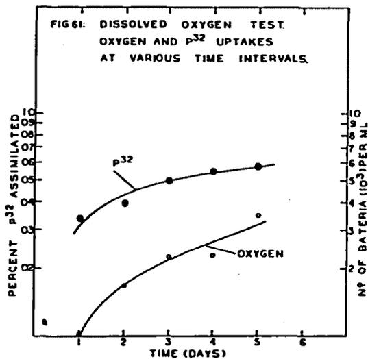
oxygen per B.O.D. bottle. This quantity is little less than 2 cc of oxygen at standard temperature and pressure. It appears that, with such a small available supply of oxygen, the proposed method of measuring the reaction rate coefficient is not adequate.
