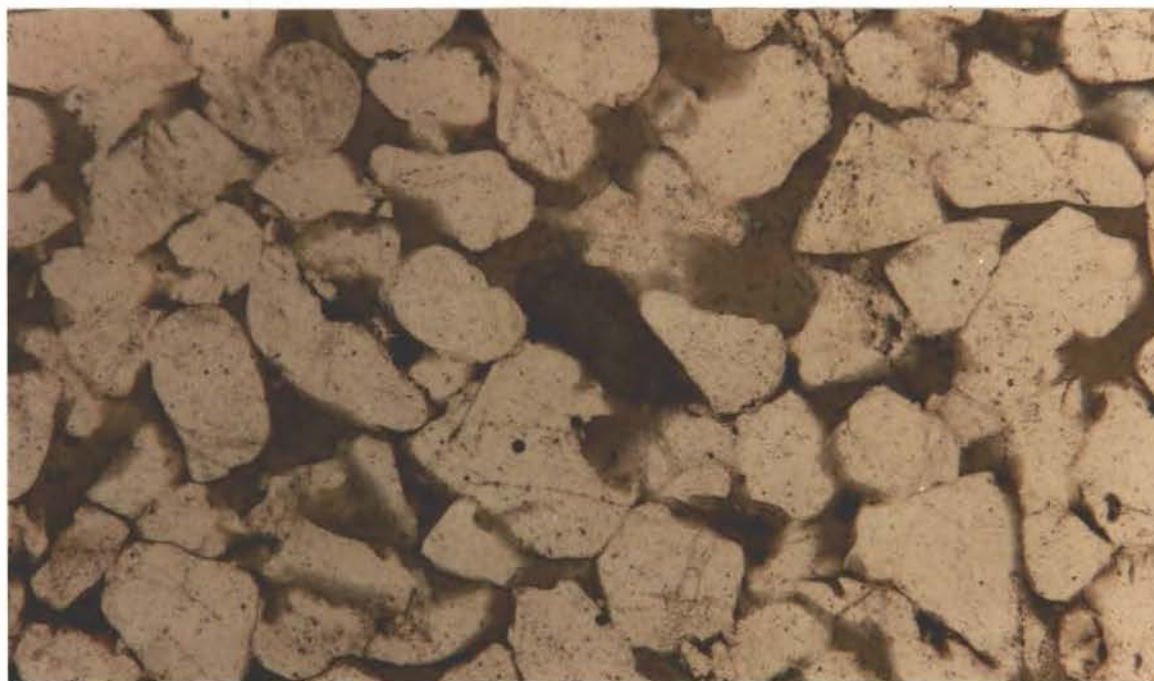
Figure 21 A) Chamosite as oolitic coatings on quartz grains (Tenneco Arkansas Kraft No.1, 13,855'). B) Chamosite as pore filler and pellets (Shell Jankowsky No.1-32, 9,812').
