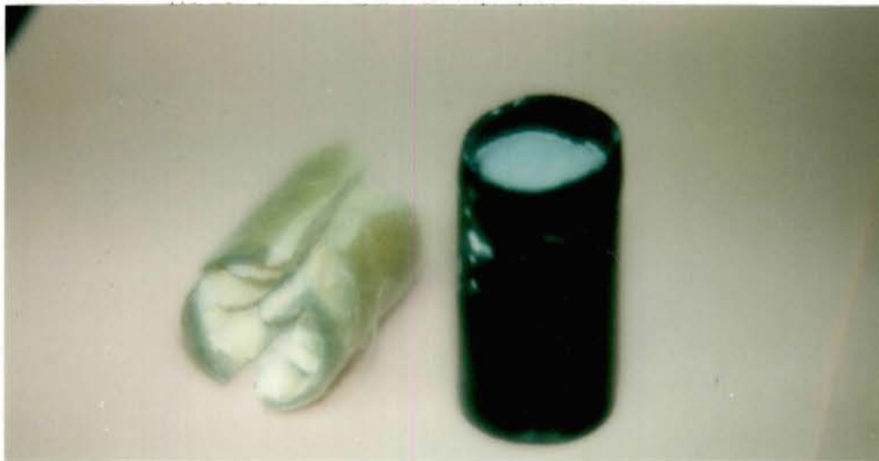
Figure 38. Limestone After 1500 PSI was Applied to the Long Axis
