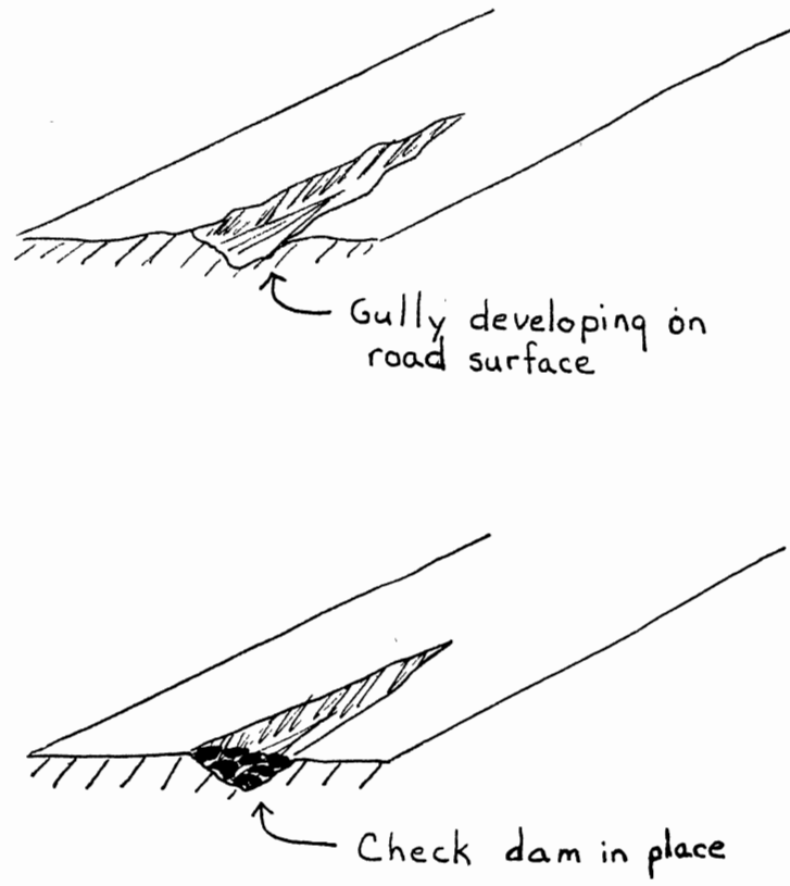
Figure 3. Check (Rock) Dam
