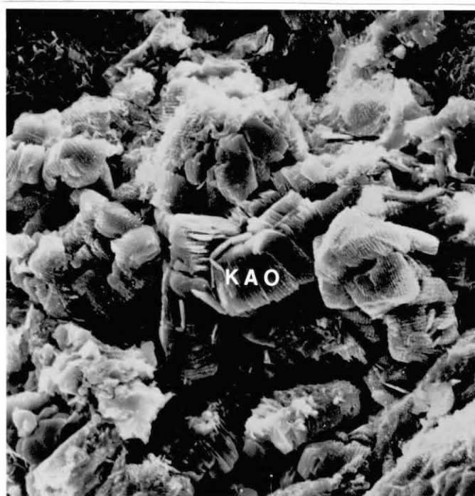
Figure 30. Microporosity In Between Kaolinite Booklets (SEM), 2500X
