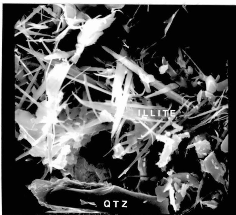
Figure 25. "Lath-like" Structures of Illite (SEM), 3000X
