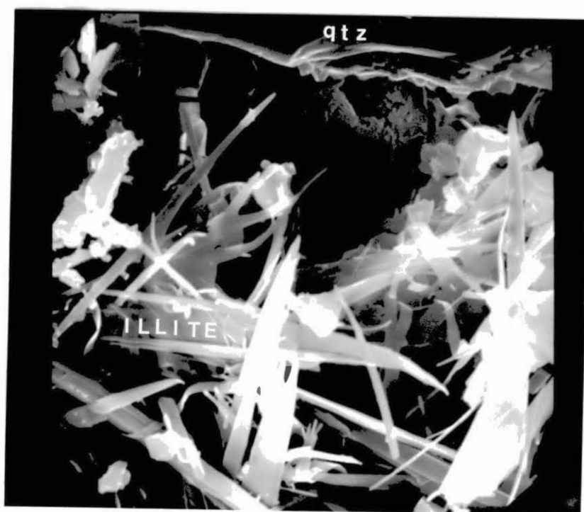
Figure 31. Illite Forming Pore Bridges Between Sand Grains (SEM), 3000X
