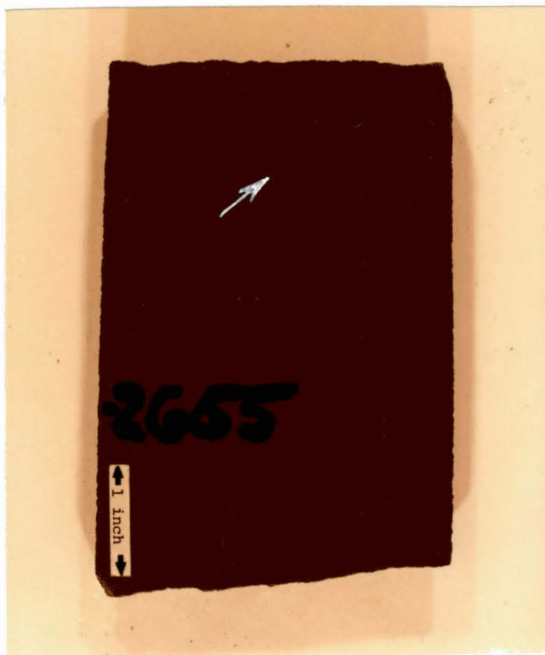
Figure 10. Horizontal or Planar Bedding, Thompson- Tye Drilling, No. 3 Shields, Depth 2655 feet, Sec. 2-T21N-R5E
