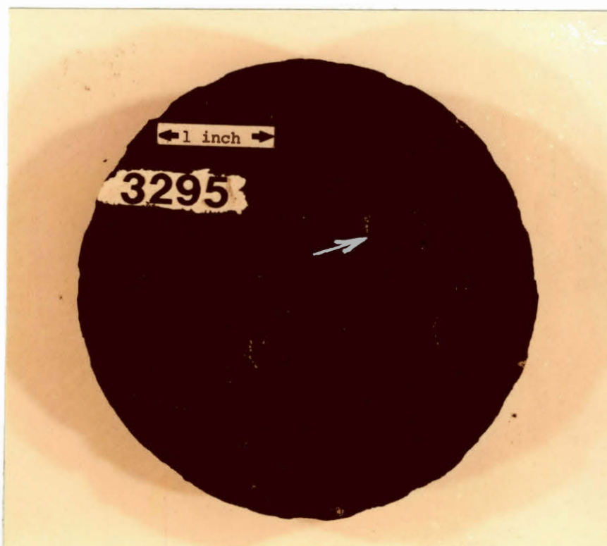
Figure 14. Fragments of Fossils in Black Shale. Brachiopod Shell in Upper Right-hand Part of Photograph. Bandera Energy Company, No. 1-8 Martin, Depth 3295 feet, Sec. 8-T22N-R5E
