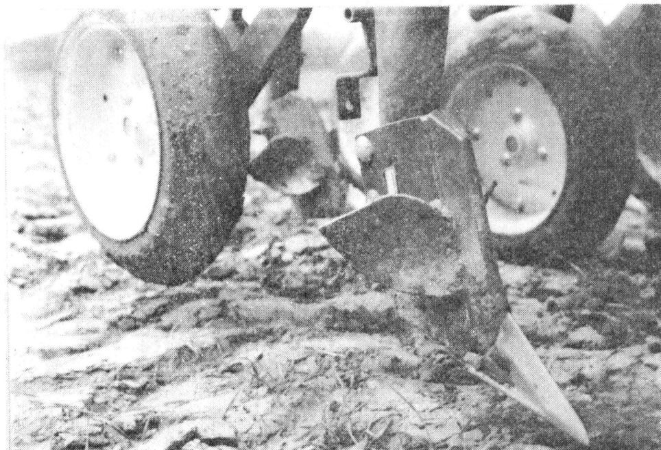
Fig. 14. 5.0 cm winged hoe used to remove treated soil, with Vee press wheel to firm seed bed.
