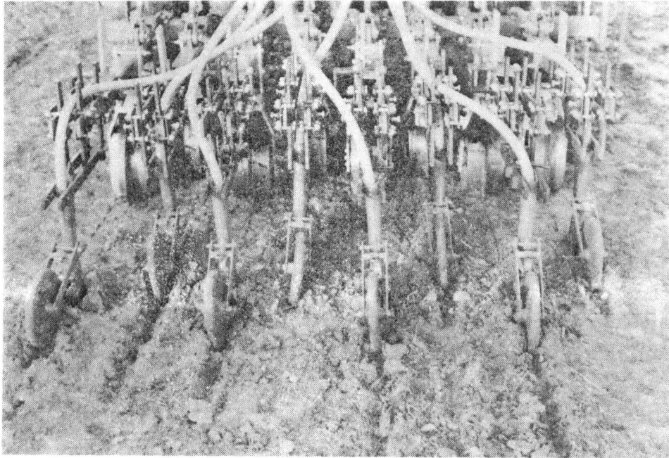
Fig. 22. 46 cm gauge coulters and hoe openers on 25 cm row spacings with 2.5 cm by 25 cm press wheels.
