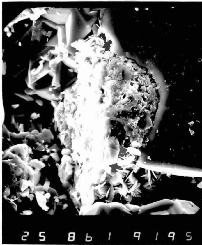
Figure 16. Dissolution of Quartz Grain, Texas Pacific #1 Shafer Depth 9.195. Magnification 860X.
