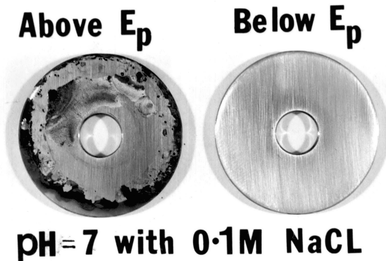
Figure 16(b). Photograph of 304 Stainless Steel exposed for 7 days in 0.1M NaCl Solution, Temp. = 80°C
