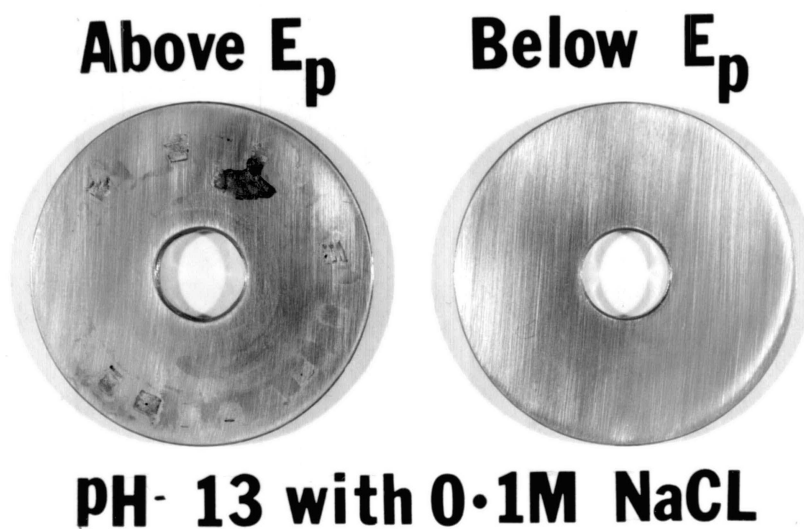
Figure 18(b). Photograph of 304 Stainless Steel exposed for 7 days in 0.1M NaCl solution, Temp. = 80^\circ\text{C}
