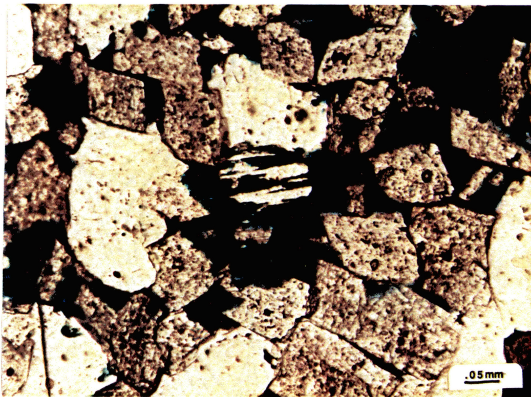
Figure 21. Photomicrograph of a Partially Dissolved Feldspar Grain (F) in the Misener Sandstone; Plane Polarized
