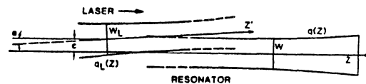
Fig. 2. Misaligned system: The laser's optical axis z' is offset by \epsilon and tilted by \alpha against the resonator's optical axis z . In this figure the waists of laser and resonator are at the same z and equal in size.
