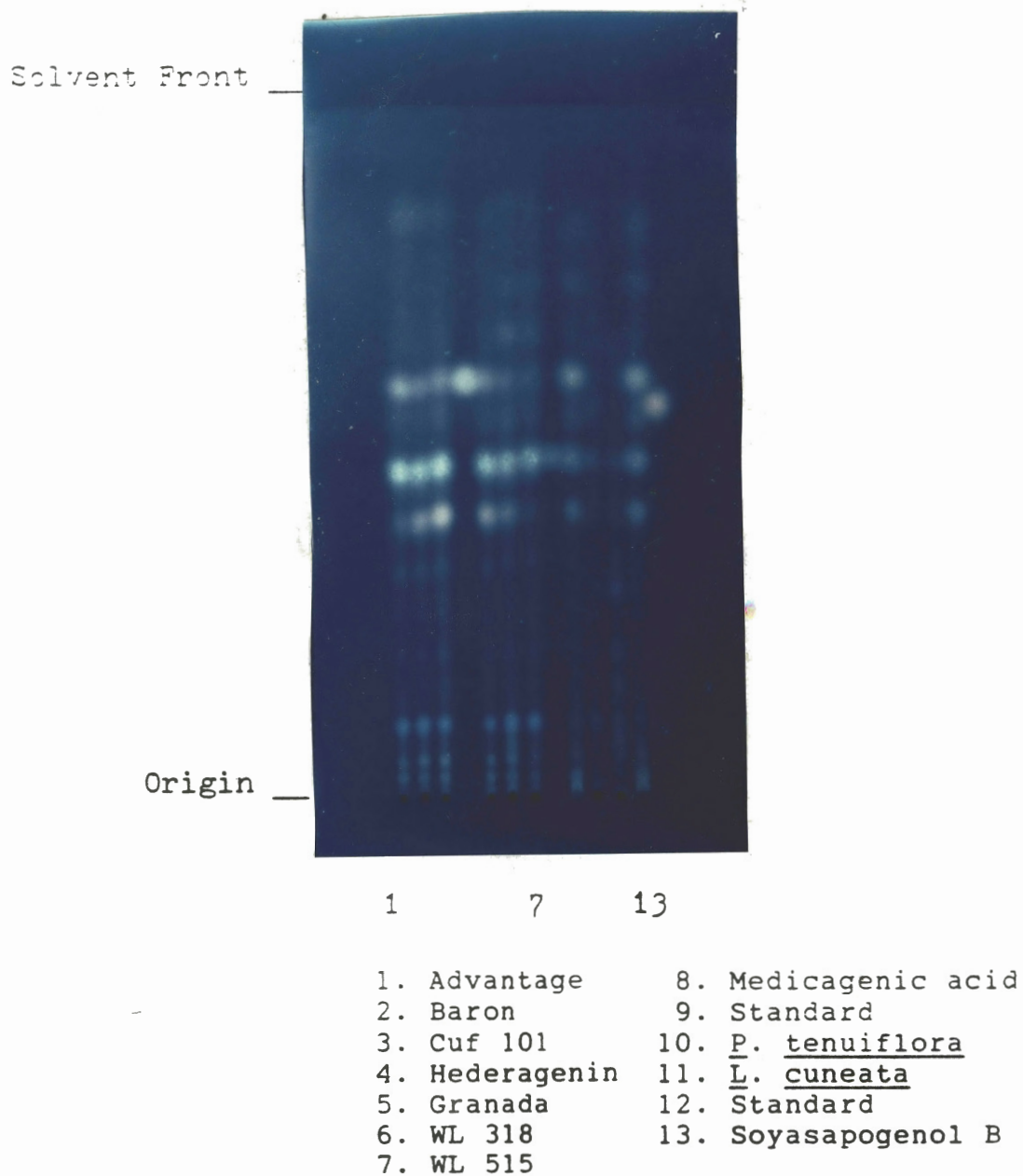
Figure 24a. Photograph of a Thin Layer Chromatogram of Alfalfa Root Aglycones from the Acid-Hydrolyzed May Samples and Standards Developed in Petroleum Ether:Chloroform:Acetic Acid 7:2:1 as Seen Under UV Lights.
