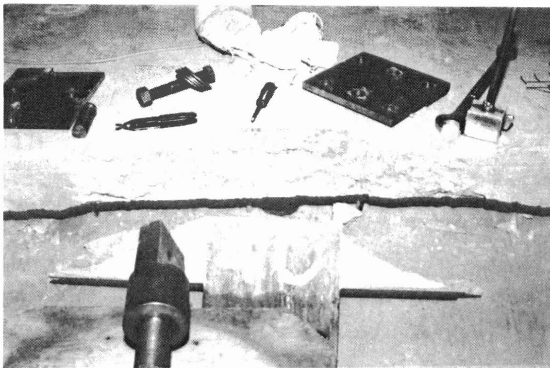
Figure 15a Failure Pattern for Type I Specimens Embedded in "Thin" Slabs
