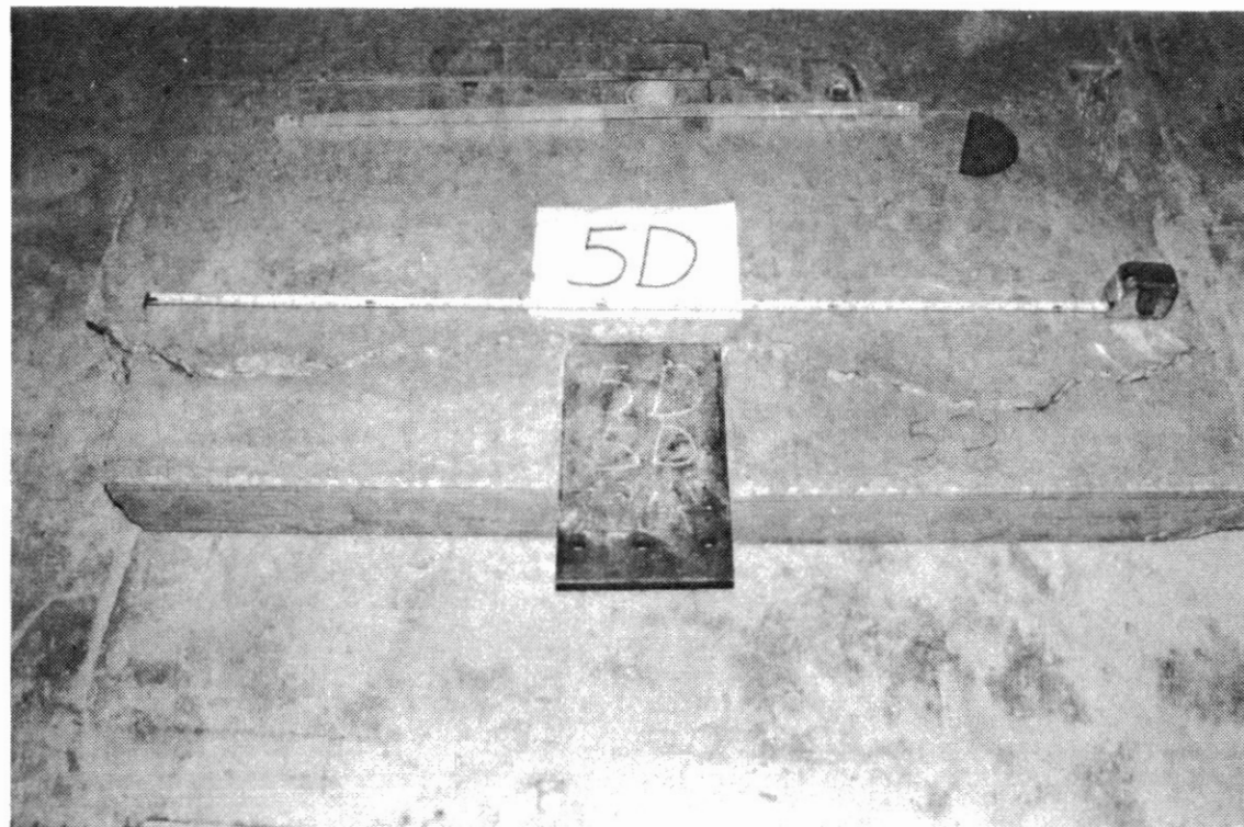
Figure 15b Failure Pattern for Type I Specimens Embedded in "Thin" Slabs
